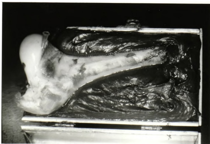
Figure 16. Bovine Femur Mold
