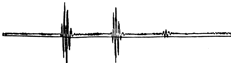
Figure 4.1.7 The waveform reflected from water/plexiglass interface
