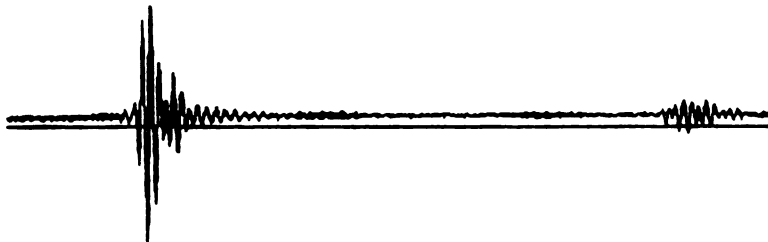
Figure 4.1.10 The waveform reflected from water/rubber interface
