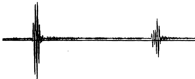
Figure 4.1.6 The waveform reflected from water/aluminum interface
