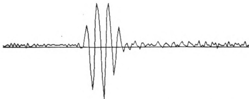
Figure 3.2.2 The waveform(2) reflected from water/aluminum interface
