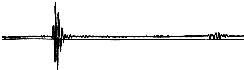
Figure 4.1.8 The waveform reflected from water/composite material interface
