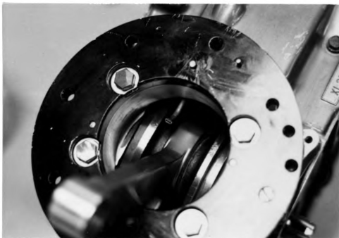
Figure 17. Line to spray oil on the connecting rod and piston bottom.
