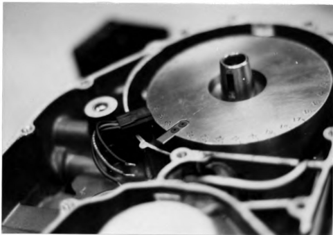
Figure 11. Flywheel with magnetic pick-up and steel timing tab.
