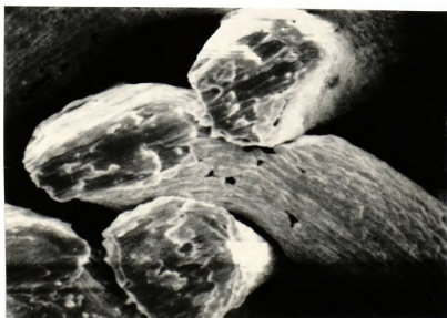
Fig. 61(b). SEM micrographs of the cross sectional area of Ag coated Cu fibers (x 500).
