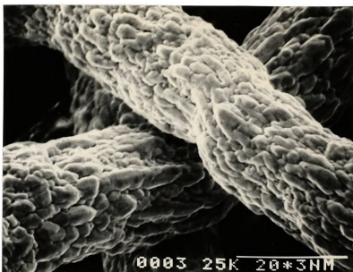
Fig. 61(a). SEM micrographs showing surface morphology of Ag coating on Cu fibers (x 1,200).
