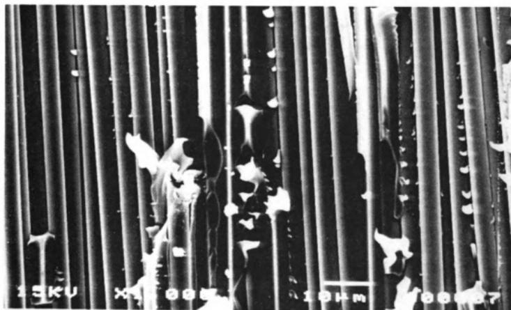
Figure 87. 1000X SEM, 100% GST sized mode II fracture.
