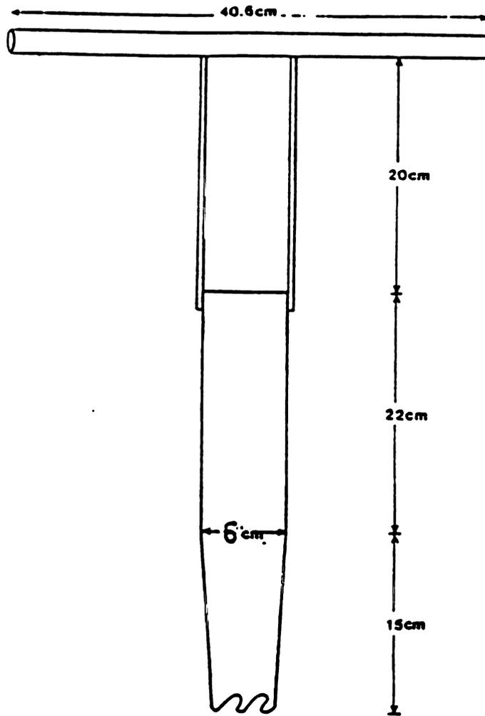
Figure 2. Diagram of soil core device.
