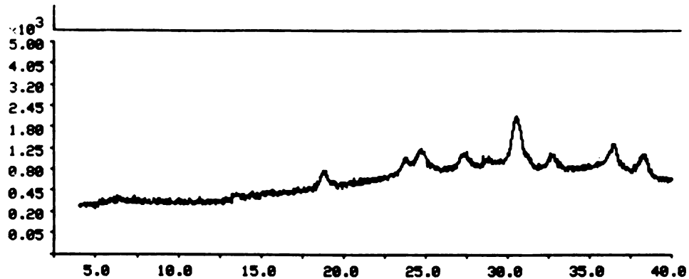
e) XRD of LDH-BCu(II)W 11 O 39 at 230°C
