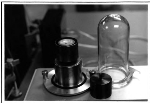
Figure 4.14a DuPont Instruments 910 Differential Scanning Calorimeter Cell (left), Showing Bell Jar (right), Cell Cover (center), and Ceramic Lid (on cell)
