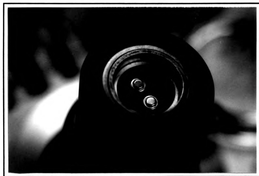
Figure 4.14b Close-up View of Sample Pan (right) and Reference Pan (left) in Calorimeter Cell Shown Above.
