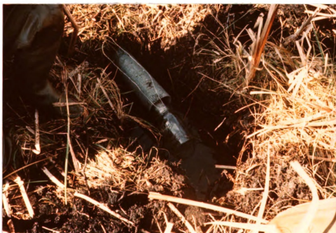
Figure 5. Design of the organic observation pits for the in-situ measurement of flow rate and collection of in-situ organic samples.
