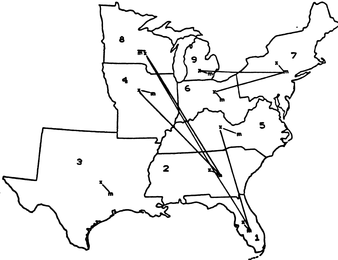
Figure 5.16. Distribution pattern under 1985 market conditions with transportation costs increased fifty percent and RO filtration applied at $.90/cwt, (TC2R09)
