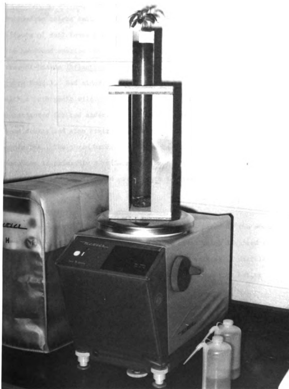
Figure 3. Soil moisture was controlled by measuring weight loss on a top-loading balance. Distilled water was added to bring weight to field capacity.
