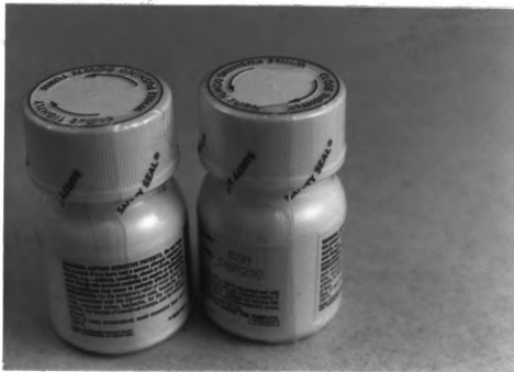
Figure 2 - The Tampered Shrink Band on the Bottle Untampered package on left, tampered package on right
