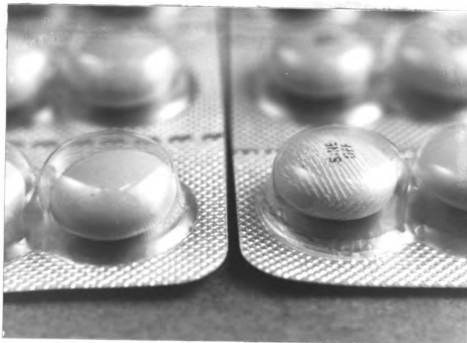
Figure 5 - The Tampered Blister Package Untampered package on left, tampered package on right
