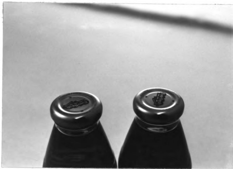
Figure 8 - Tampered Vacuum Button (View 2) Untampered package on left, tampered package on right
