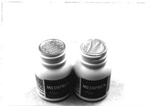
Figure 3 - The Tampered Membrane Seal Untampered package on left, tampered package on right
