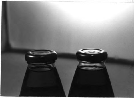
Figure 7 - Tampered Vacuum Button (View 1) Untampered package on left, tampered package on right
