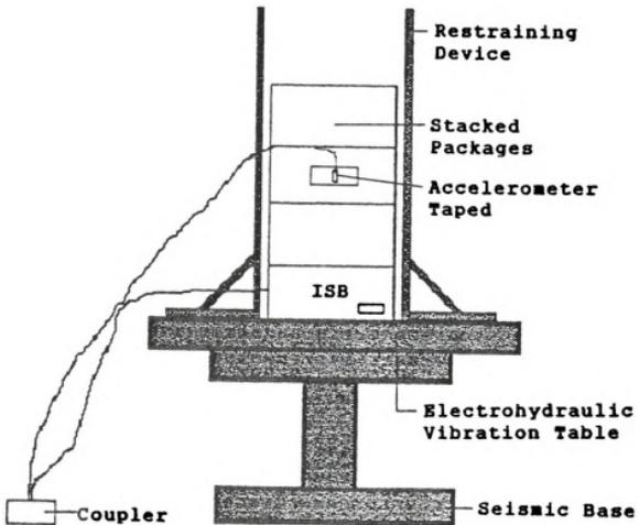
Figure 11. Test Setup for Comparing Forces and Accelerations
