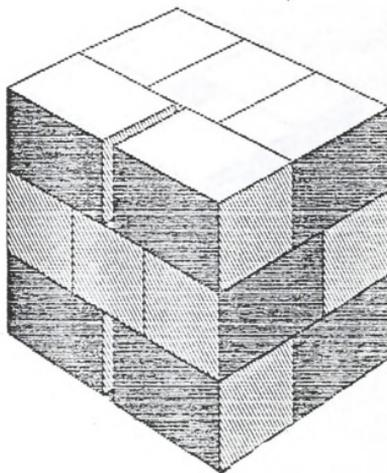
Figure 8. Interlock Type Pallet Pattern
