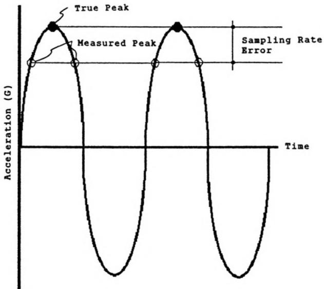
Figure 4. True Peak vs Measured Peak
