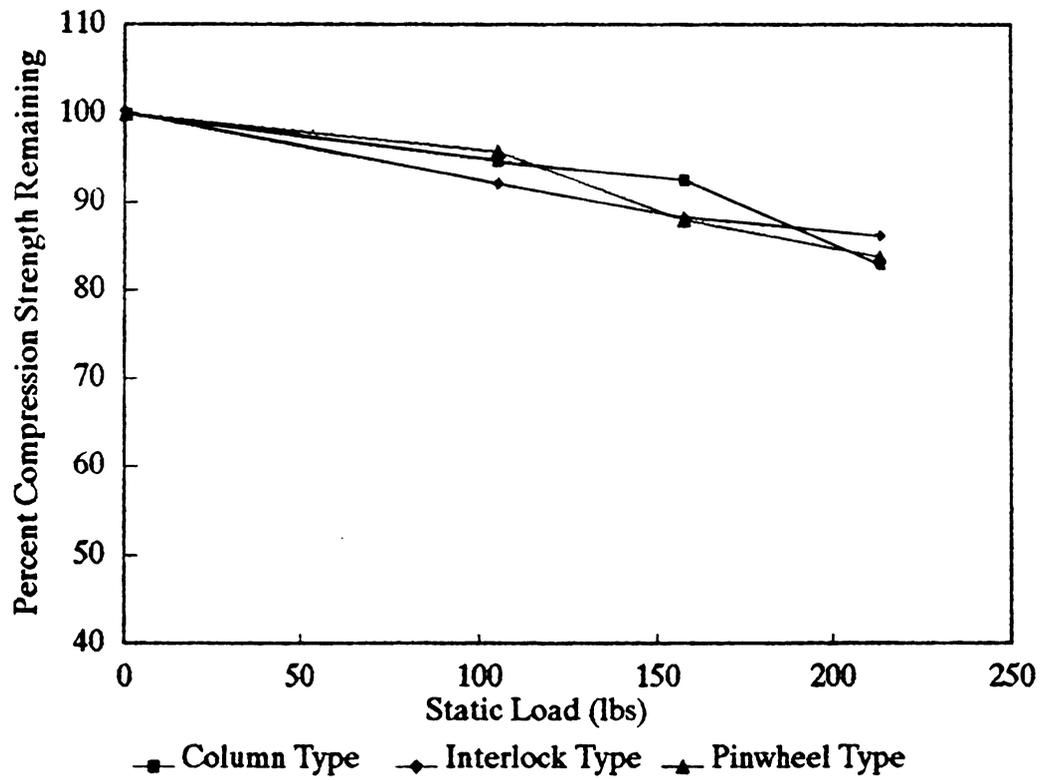
Figure 13. Mean Percent Compression Strength Remaining
