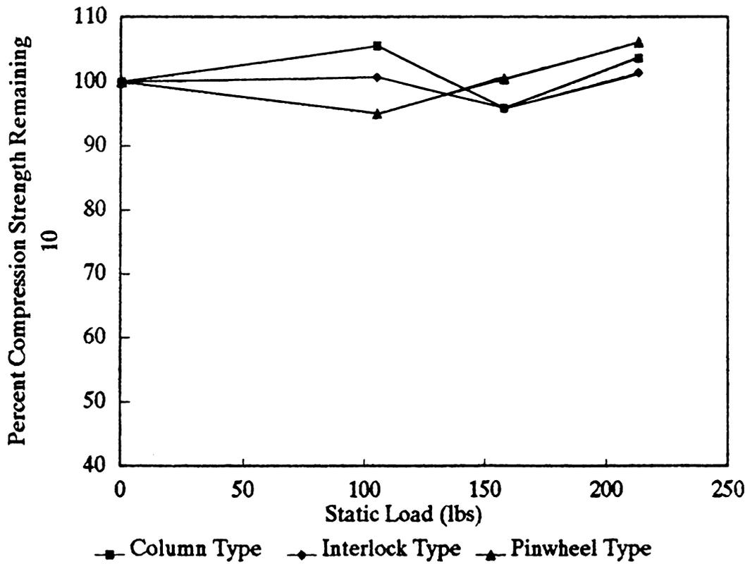
Figure 14. Mean Percent Compression Strength Remaining
