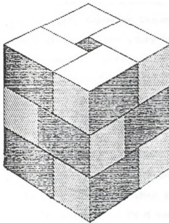
Figure 9. Pinwheel Type Pallet Pattern
