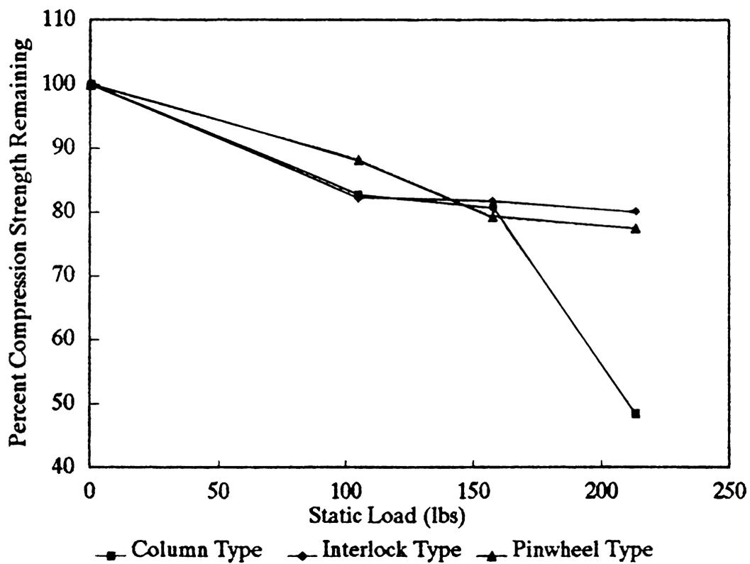
Figure 12. Mean Percent Compression Strength Remaining
