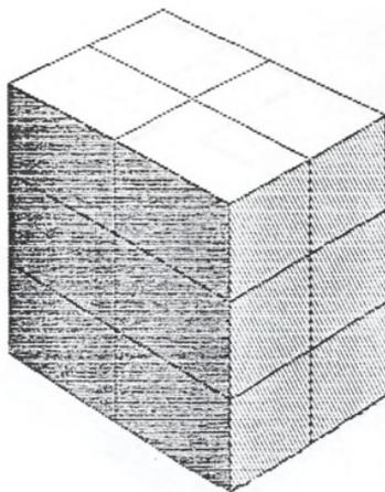
Figure 7. Column Type Pallet Pattern
