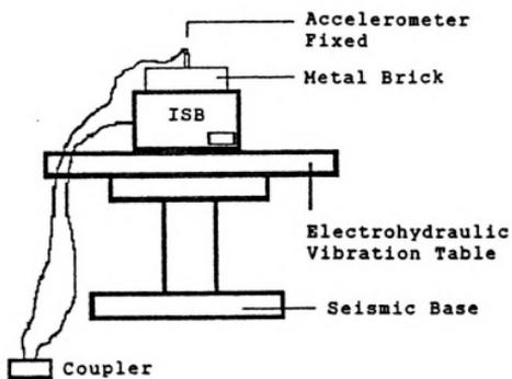
Figure 2. Test Setup for Dynamic Force Relative to Acceleration
