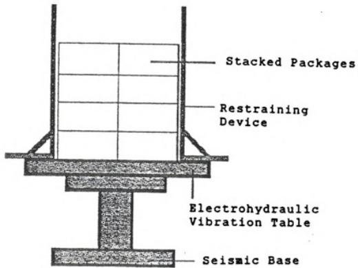
Figure 10. Test Setup for Vibration
