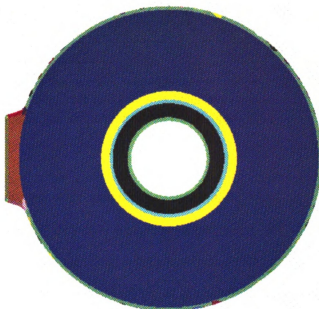
Figure 7.10. Labeling of surface regions for gear blank model exhibiting artifacts in filleted and rounded regions.
