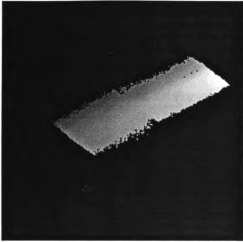
Figure 1.2. Depth map of a cylindrical casting. (Intensity coding of depth.)
