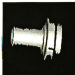
Figure 4.11. Pseudo-intensity rendering of depth map of defect-free spindle-like casting.
