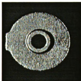
(h) Image of defect-free casting labeled "Good".
