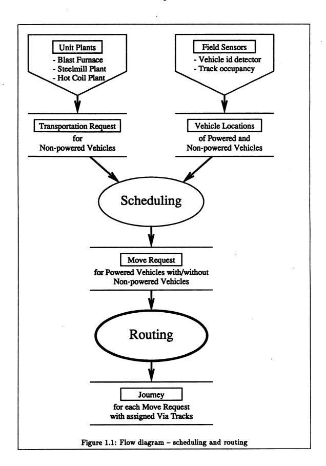
Figure 1.1 shows an example for scheduling and routing functions in a steelmill company. Each unit plant sends a transportation request to the railway control system. The scheduling function invokes moverequests using the vehicle location information for the transportation requests. Then the routing function computes the optimal route for each moverequest. We call the moverequest with an assigned route a *journey*. A formal definition of the *journey* will be given in Chapter 2.
