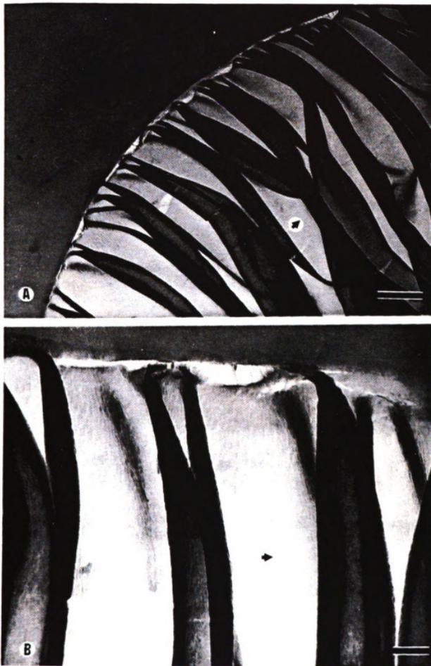
**Figure 6.4** - TEM micrographs of a radially sectioned fluorinated Kevlar-49 aramid fiber (treatment D). (A) bar = 500 nm (B) bar = 100 nm
