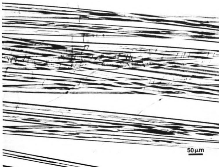
**Figure 3.13** - Optical micrograph of "as received" PBO fibers, showing presence of compressive kink bands.
