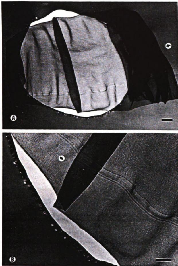
**Figure 7.5** - TEM micrographs of  $100 \text{ keV } 10^{15} \text{ Ti}^+/\text{cm}^2$  irradiated Kevlar-49 fiber. (A) whole fiber view, (B) fiber-matrix interphase. (A) bar =  $1 \mu\text{m}$  (B) bar =  $500 \text{ nm}$
