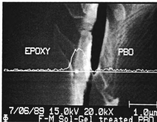
**Figure 8.7** - AES line-scan of silicon superimposed on a SEM micrograph of a Foster-Miller sol-gel treated PBO fiber imbedded in an epoxy matrix. (○ cross-sectional view).
