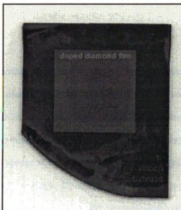
Figure 4.22. Deposited doped diamond film on the front side of sample A.
