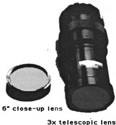
**Figure 5.3.** The 6" close-up lens and the 3x telescopic lens used to increase the spatial resolution of the radiometer.
