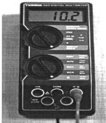
Figure 5.4. The Omega 880 Digital Multimeter.
