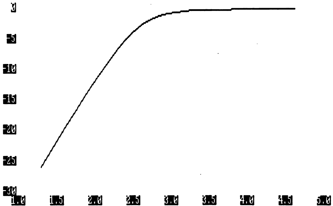
Figure 2.4 - Bode Magnitude Plot of High Pass Filter
