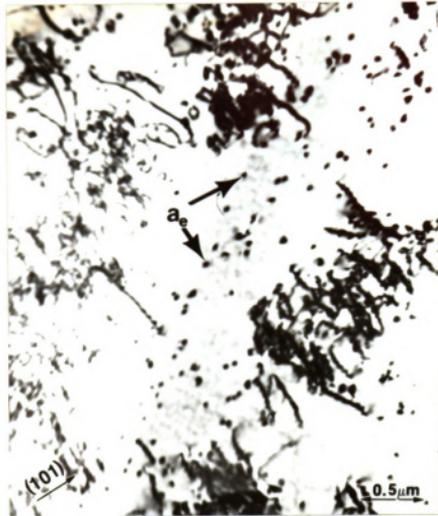
Figure 22: Diffraction contrast micrograph with foil normal of  $[010]$ . The dark spots represent dislocations with an end on configuration for imaging in phase contrast conditions. The diffracting vector is  $(101)$ .
