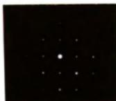
Figure 23 : (b) The same  $\{100\}$  zone with an objective aperture to limit the number of diffracted beams for phase contrast imaging.
