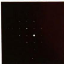
Figure 23 : (a) Diffraction spot pattern of a single crystal thin foil of Ni-50Al, showing a  $\{100\}$  zone for the B2 crystal structure with no objective aperture. The additional diffraction spots are created from the superlattice.
