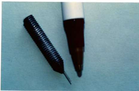
Figure 27. Needle probe for thickness measurements.
