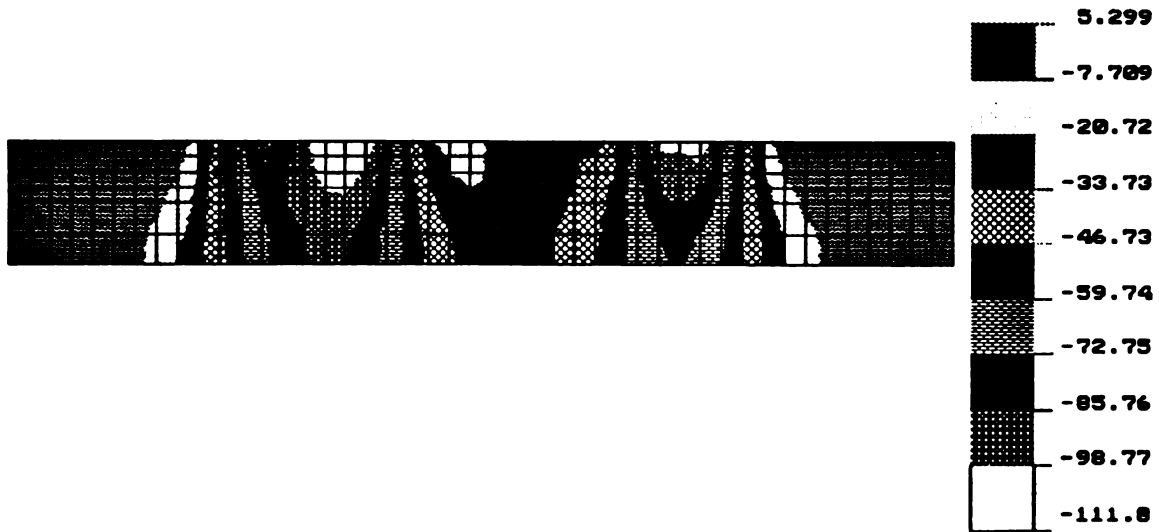
Figure 52. Homogeneous FEM, stresses normal to surface.
