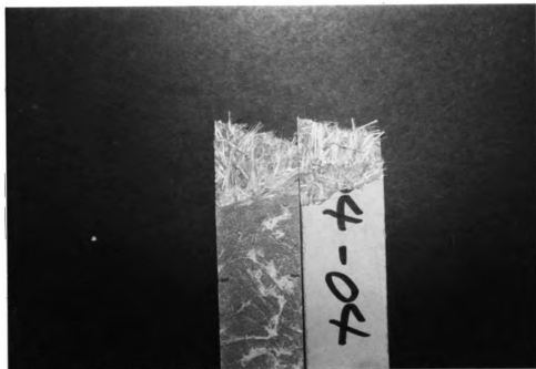
Figure 4.17 Fractured Surface-Unaged GFRC.
