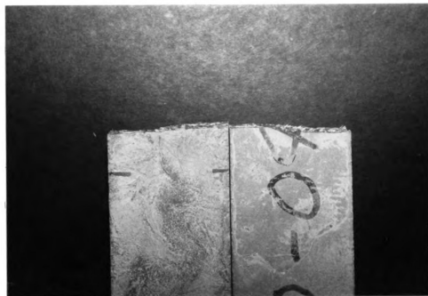
Figure 4.32 Fractured Surface-Aging in Hot Water.
