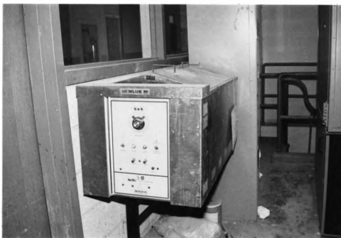
Figure 3.2 Water Bath for Accelerated Aging.
