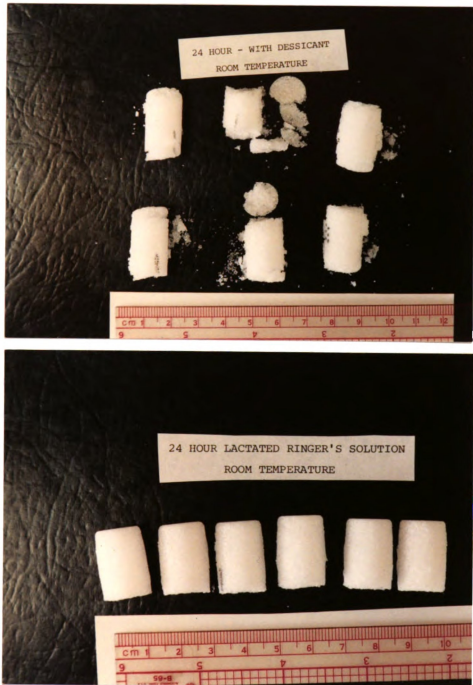
FIGURE 5: Results showing the contrast between modes of failure of "dry" HTR® plugs and those soaked in lactated ringers solution. This graphic demonstration prompted an experiment to analyze how much fluid molded HTR® would absorb.
