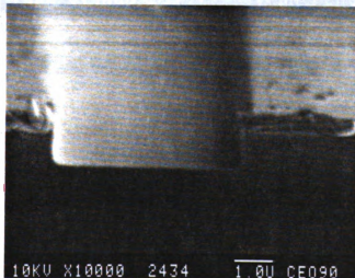
Figure 5.1 a) sub-micron, b) 3\mu\text{m} , and c) 5\mu\text{m} wide trenches etched in silicon (0.7 mTorr, 600 Watts Microwave Power, -50 volts, L_s=21.5\text{cm} , L_p=1.4\text{cm} )
