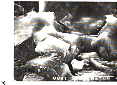
Figure 22. Scanning electron micrographs of the fracture surface of Macor specimen MA-9. a) view at edge of fracture surface, 750 X, b) view of fracture surface near tensile surface, 3000 X.
