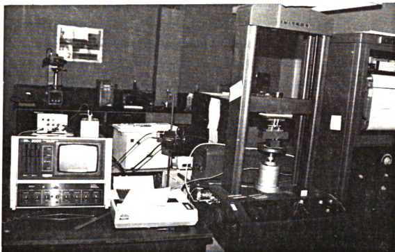
Figure 15.a. Photograph of fatigue - AE experimental station.
