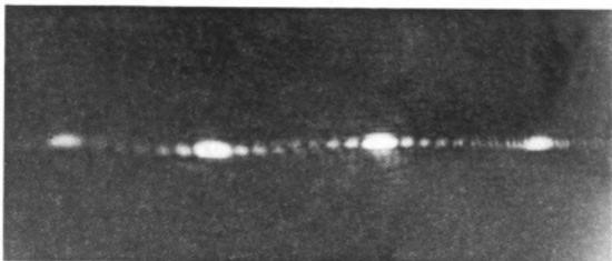
Figure 2.5. Beam divider diffraction patterns with a Helium-Neon laser.
