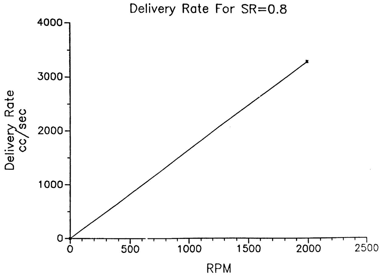
Figure B1. Delivery rate vs. RPM for a 124cc engine with SR=0.8.
