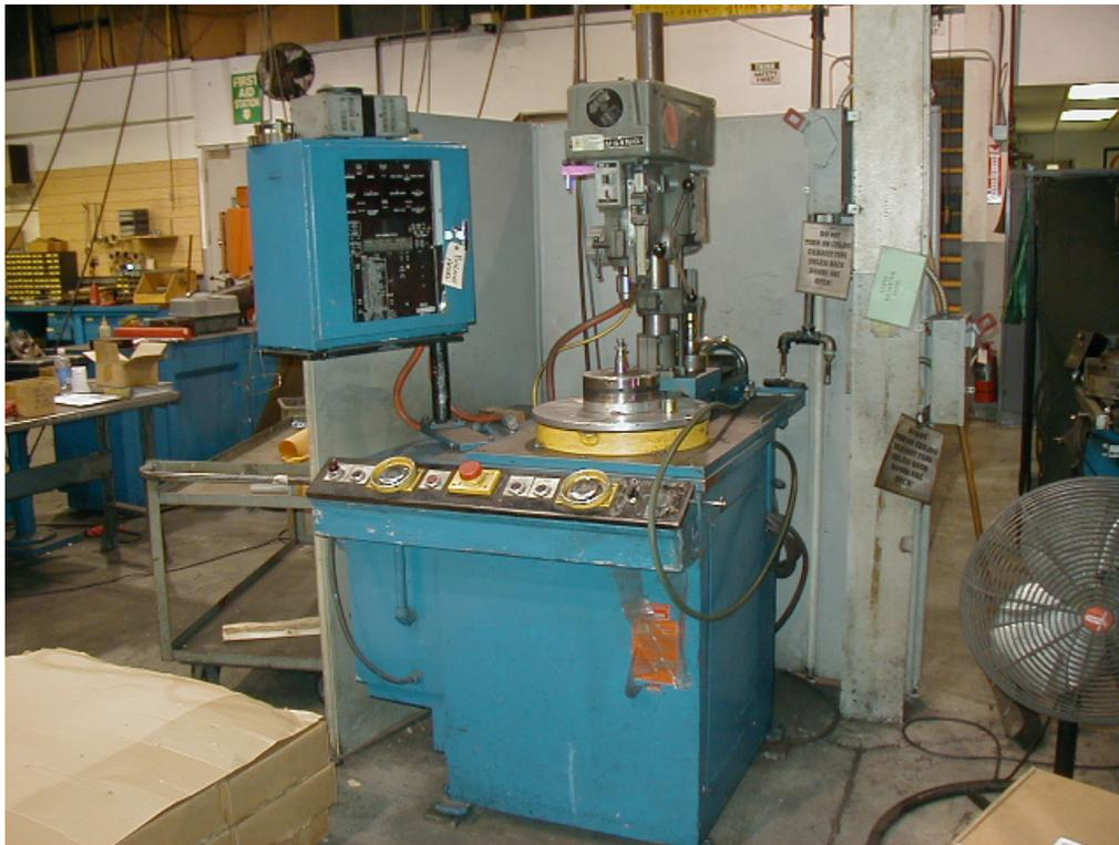
*Figure 17: Balance Engineering Corporation automatic balance machine.*
