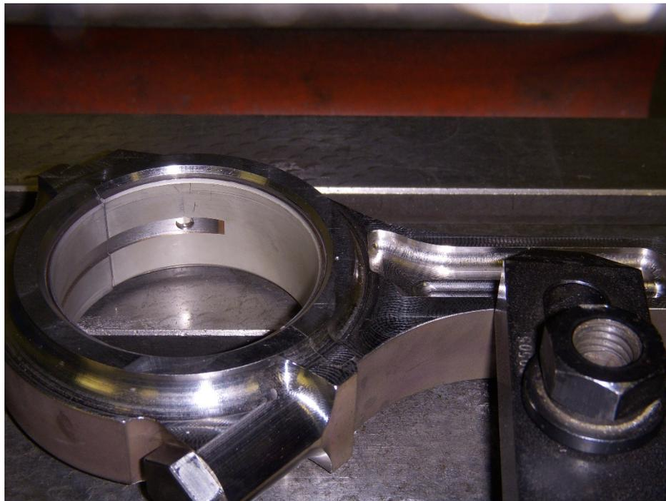
*Figure 20: A Connecting rod mounted on a mill to measure the mark made by balancing it on a pin.*
