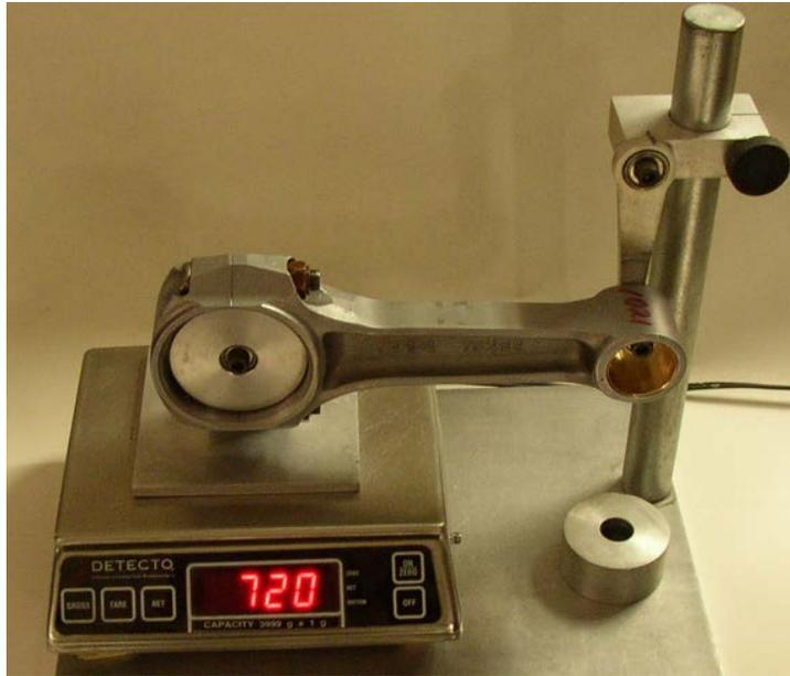
*Figure 21: A connecting rod being weighed to find the large and small end weights.*
