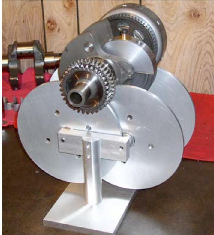
*Figure 19: Crankshaft mounted on a static balance stand.*
