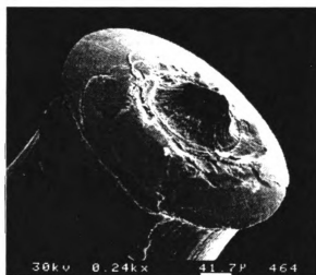
Figure 2.9 SEM pictures of STM tips. (a) cut Pt-Rh tip. (b) pulled Nb tip.
