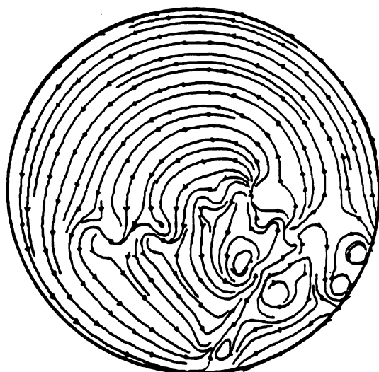
Figure 31. Streamlines and velocity profiles at y=0 as a function of time (without swirl). Injector at 60 degrees (counterclockwise from horizontal). U_{in} = 210.0 m/s.
