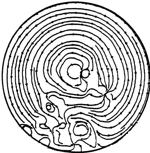
Figure 41. Streamlines and velocity profiles at y=0 as a function of time (with swirl). Injector at 120 degrees (counterclockwise from horizontal). U_{in} = 210.0 m/s.
