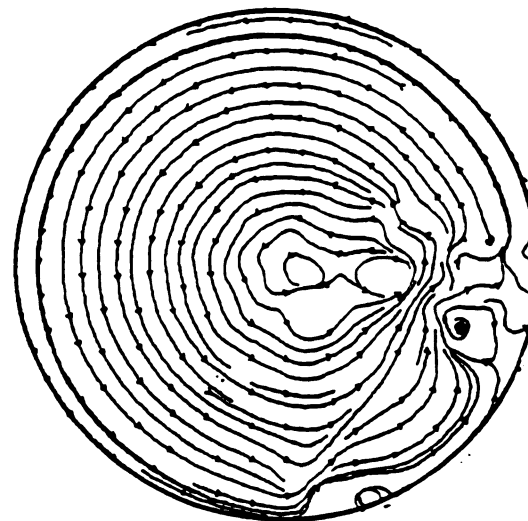
Figure 33. Streamlines and velocity profiles at y=0 as a function of time (with swirl). Injector at 60 degrees (counterclockwise from horizontal). U_{in} = 210.0 m/s.
