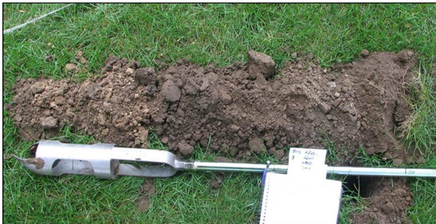
Figure 15. Soil core auger:
