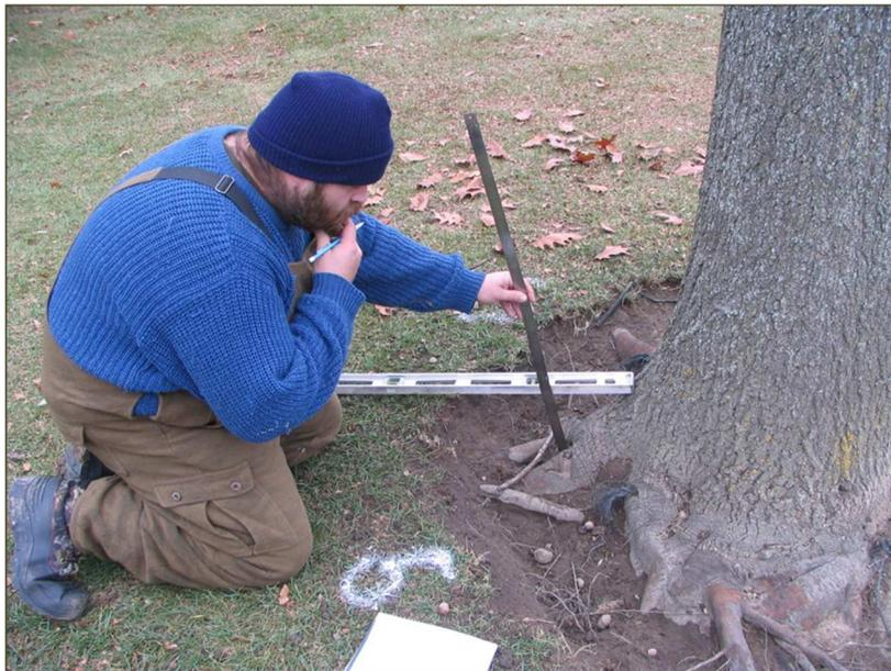
Figure 12. Measuring depth of original root flare (DORF) at site AD: Demonstration of the technique used to measuring depth of original root flare.
