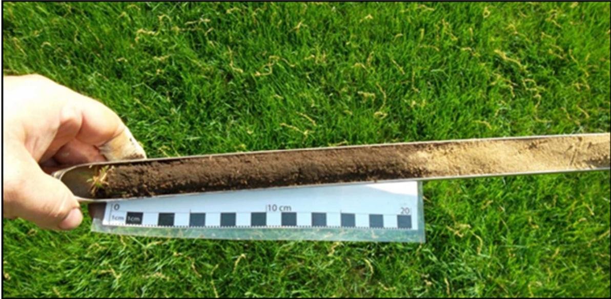
Figure 16. Cores to determine top soil depth:
