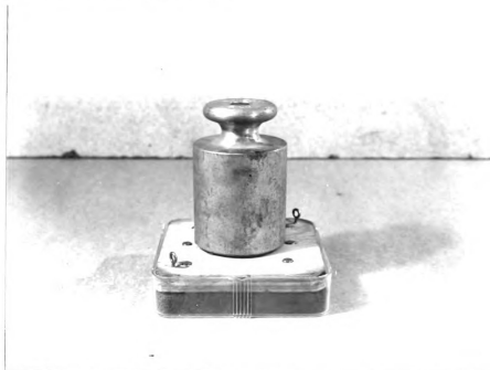
Fig. 3. Soil being compacted with a five-pound weight.
