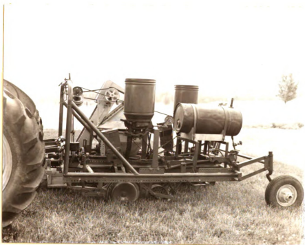
Fig. 19. Field planter with remote hydraulic cylinder removed.
