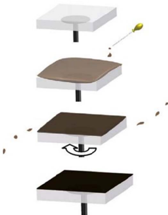
Figure 1.1 Illustration of the spin-coating technique for forming polymer thin films. The film becomes thinner as the substrate rotates to bring the polymer solution to the edge, and eventually a uniform thin film forms on the substrate.
