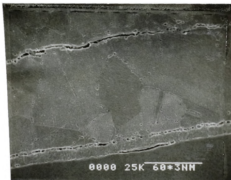
FIG. 19. SEM micrograph of an Cu-Hi composite tensile specimen annealed at 750 C for 5 minutes (just below fracture surface).
