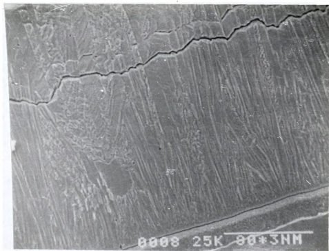
FIG.17. SEM micrograph of transverse section of unannealed Cu-Ni composite tensile specimen (below fracture surface).
