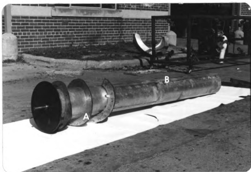
Fig. 4 Photograph of the rotor: A. Auger flighting; B. Straight paddles.
