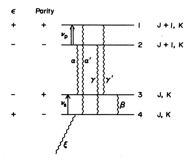
Figure 1. Energy level scheme for a four-level double resonance experiment in  $\mathrm{NH}_3$ .
