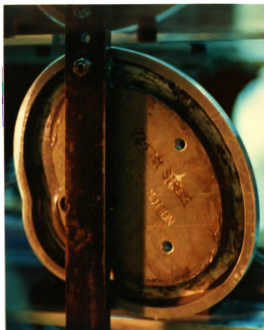
Figure A.1: (a) The differences between the piston motion of a normal four-stroke engine and the water analog model used in this work. The differences, required because of incompressibility of water, are also shown in phase space. (b) A picture of the cam-shaft used to create the piston motion.
