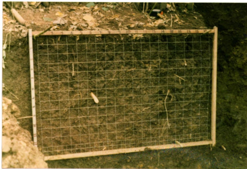
Figure 4.2. The rectangular counting frame that was used in counting roots within a profile. The frame had a depth of 60.9 cm and a length of 96.5 cm.
