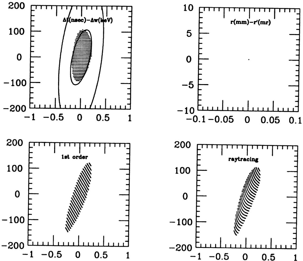
Figure 5.10: The phase space transformations of the longitudinal linear acceptance in the system using solenoids for the transverse focusing. The incident velocity of the  $^{238}\text{U}^{24+}$  beam was  $0.0085c$ .
