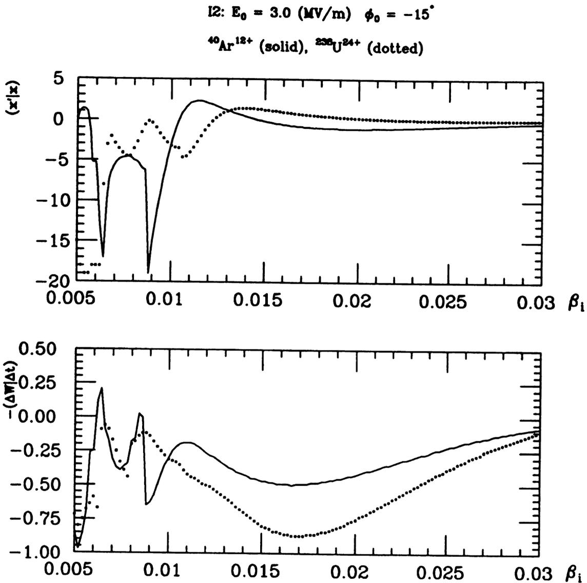
Figure 4.8: The plots of  $(x'|x)$  and  $-(\Delta w/\Delta t)$  vs. initial beta  $\beta_i$  for an I2 type resonator. The solid line is for  $^{40}\text{Ar}^{12+}$  and the dotted line is for  $^{238}\text{U}^{24+}$ .
