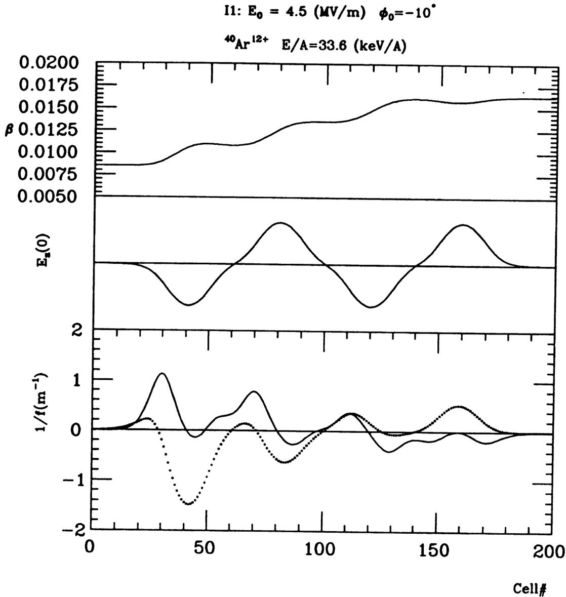
Figure 4.3: The focusing power at each cell of an I1 type resonator for  $^{40}\text{Ar}^{12+}$  beam with initial value of  $\beta = 0.0085$  (bottom). The solid line is for transverse direction and dotted line is for longitudinal direction. The top shows the  $\beta$  profile along the resonator axis. The middle part is an axial electric field profile of the I1 type resonator which has a four gap structure.
