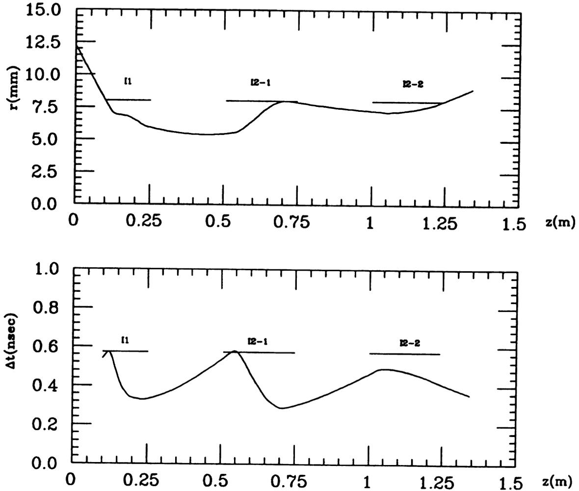
Figure 5.2: The beam envelopes of beam radius (upper) and deviation of time of flight (lower) starting from maximum emittance.
