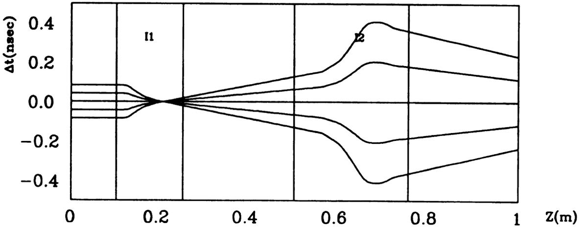
Figure 4.14: The longitudinal raytracing plots for  $^{40}\text{Ar}^{12+}$  (up) and  $^{238}\text{U}^{24+}$  (down) beams with parallel rays ( $\Delta W = 0$ ) at the beginning.
