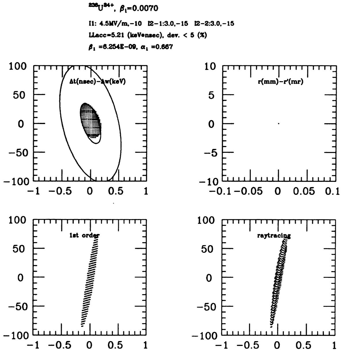
Figure 5.5: The phase space transformations of the longitudinal linear acceptance for a  $^{238}\text{U}^{24+}$  beam with an incident velocity  $0.007c$ .
