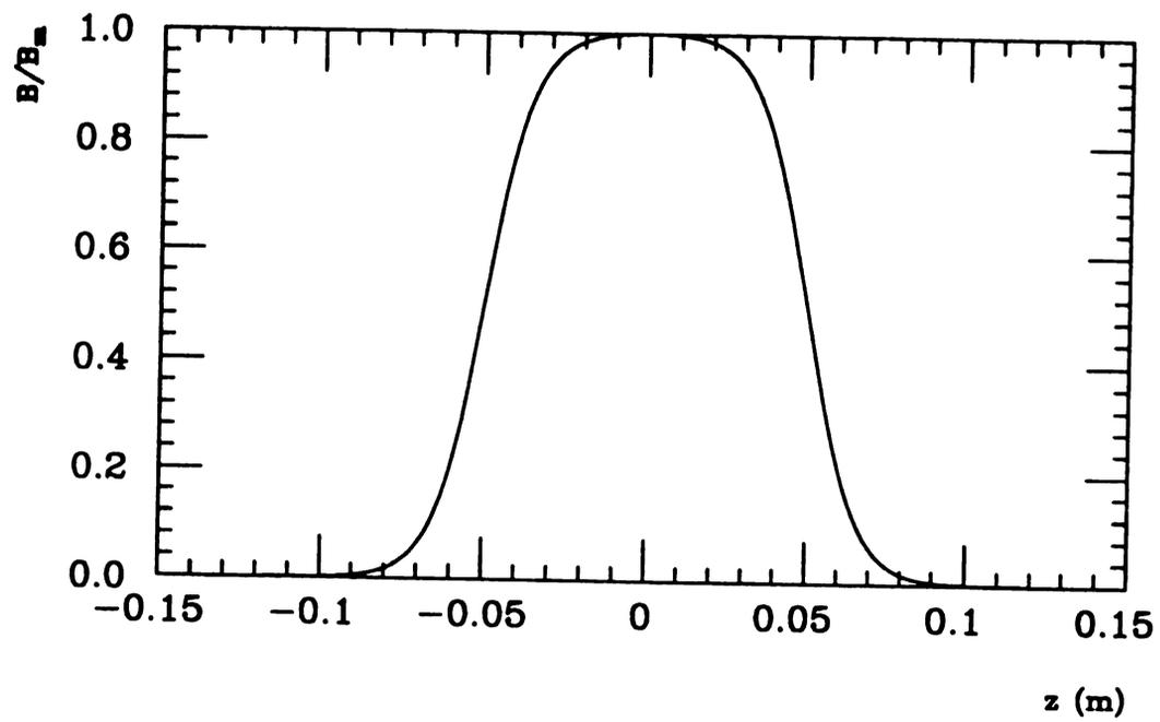
Figure 3.1: The normalized magnetic field profile on axes of the model solenoid with half aperture 1.5 cm and body length 10 cm.
