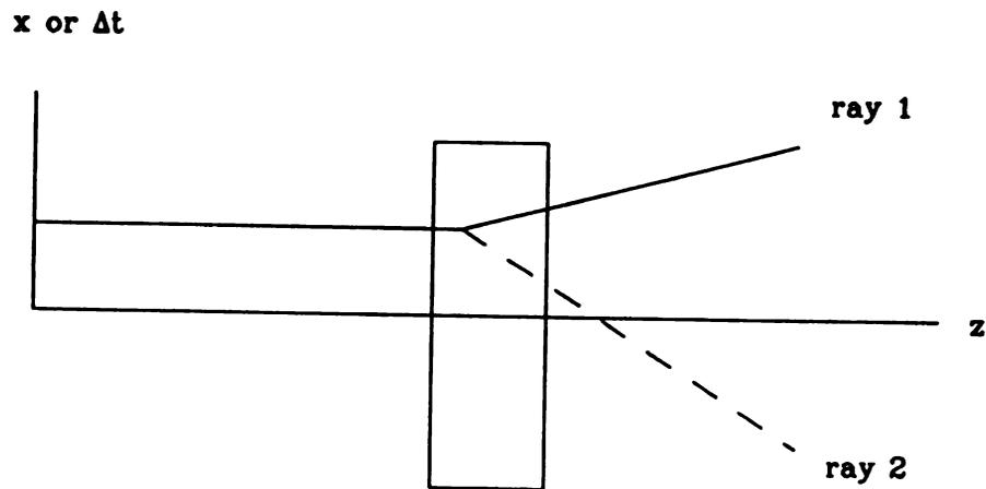
Figure 4.2: The focusing and defocusing actions of a lens.  $(x'|x)$  or  $-(\Delta w|\Delta t)$  is positive for ray 1 to give net defocusing action and negative for ray 2 to give net focusing action
