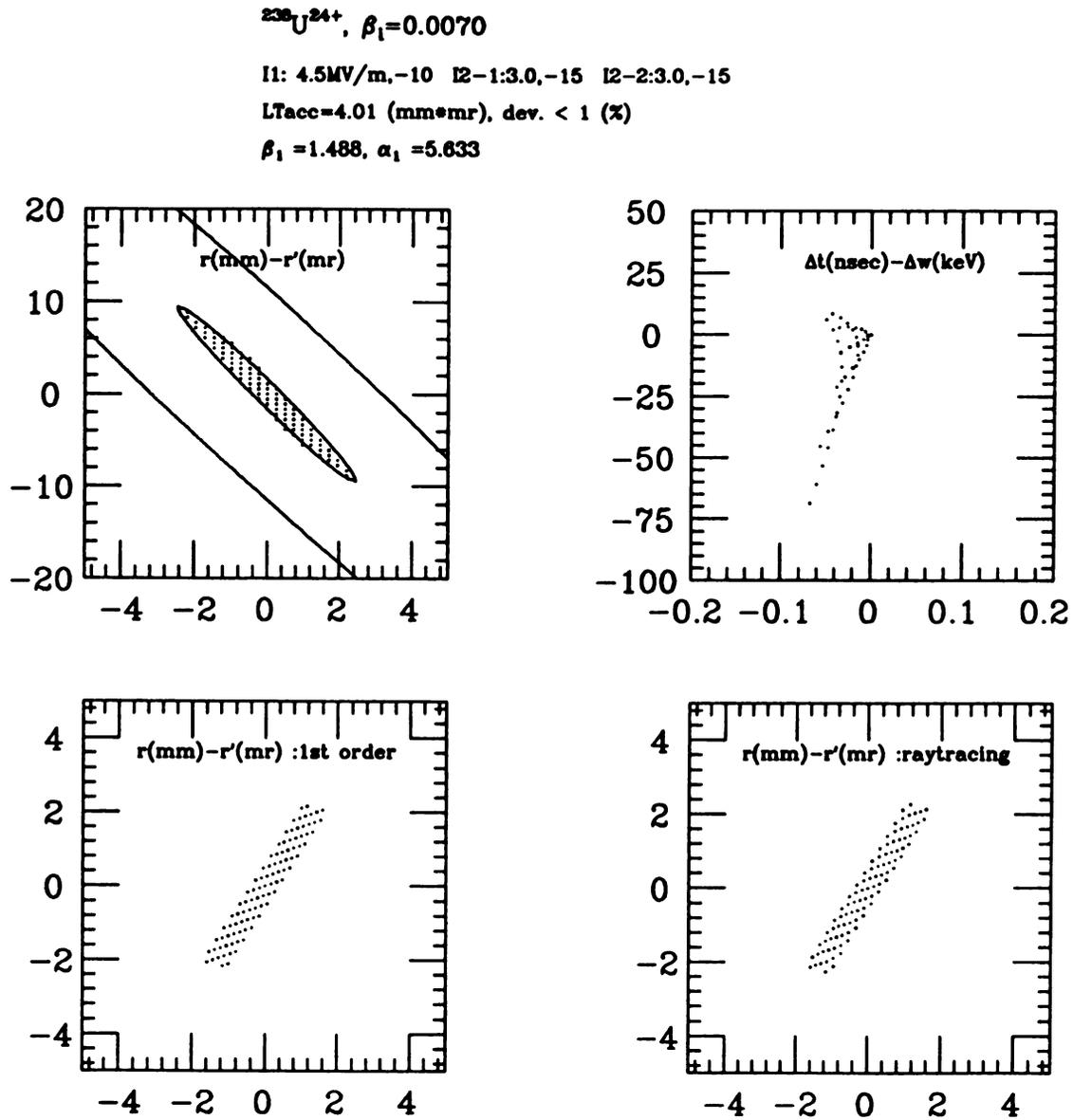
Figure 5.3: The phase space transformations of the transverse linear acceptance for a  $^{238}\text{U}^{24+}$  beam with an incident velocity of  $0.007c$  and with a deviation of 1%.
