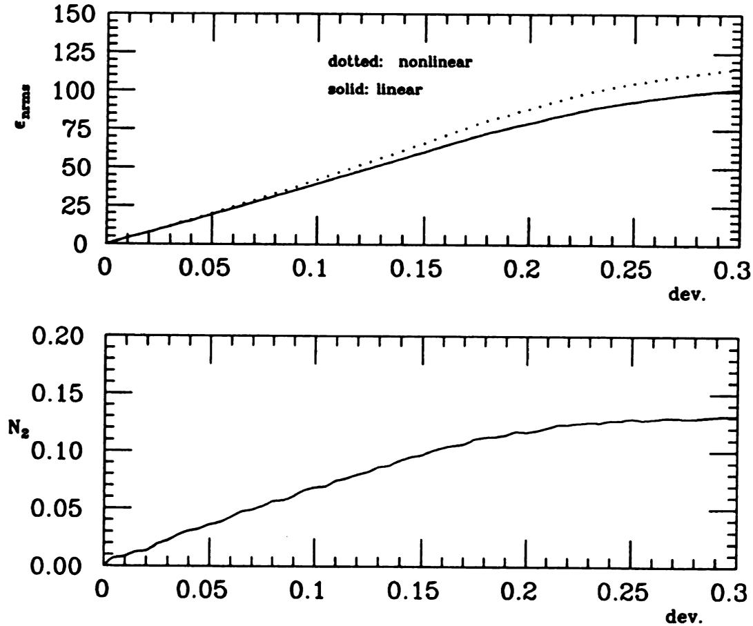
Figure 5.12: The relationship between scalings of nonlinearity by linear transformation and by rms emittance for a  $^{238}\text{U}^{24+}$  beam with an incident velocity 0.0085c in the system using solenoids for transverse focusing. The initial geometrical longitudinal acceptance was 117.4 keV·nsec without transverse phase space.
