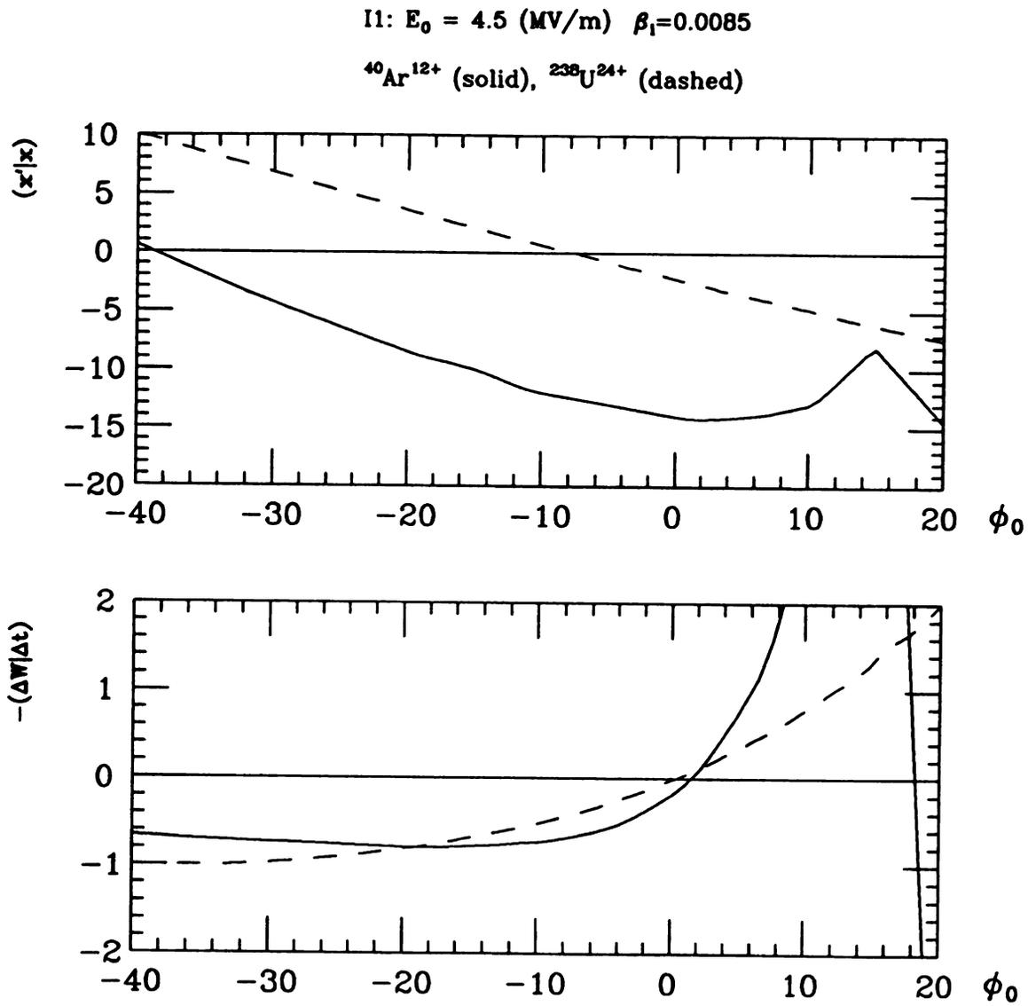
Figure 4.9: The plots of  $(x'|x)$  and  $-(\Delta w|\Delta t)$  vs. rf phase offset  $\phi_0$ , for an I1 type resonator. The solid line is for  $^{40}\text{Ar}^{12+}$  and the dashed line is for  $^{238}\text{U}^{24+}$ .
