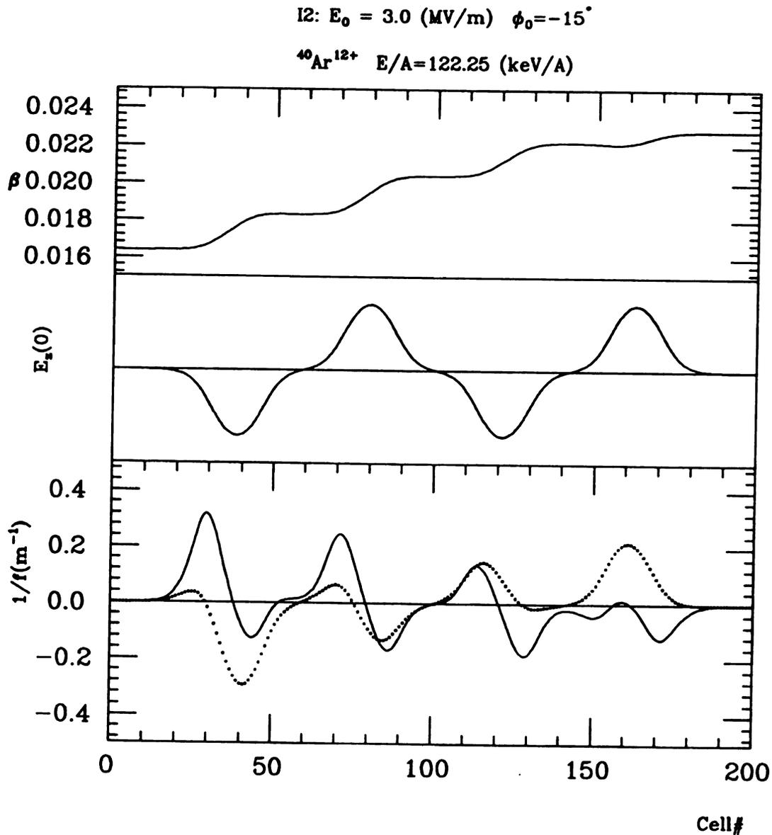
Figure 4.4: The focusing power at each cell of an I2 type resonator for  $^{40}\text{Ar}^{12+}$  beam with initial value of  $\beta = 0.0164$  (bottom). The solid line is for transverse direction and dotted line is for longitudinal direction. The top shows the  $\beta$  profile along the resonator axis. The middle part is an axial electric field profile of the I2 type resonator which has a four gap structure.
