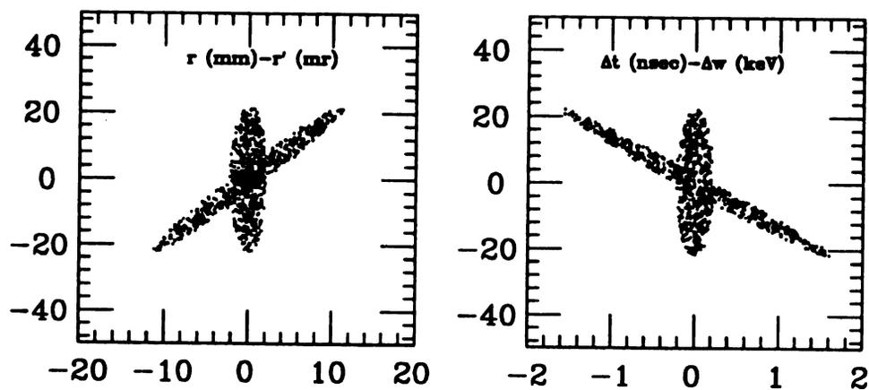
Figure 1.5: The actions of drift space on the transverse (left) and the longitudinal (right) phase spaces. The initial phase space ellipses are upright.
