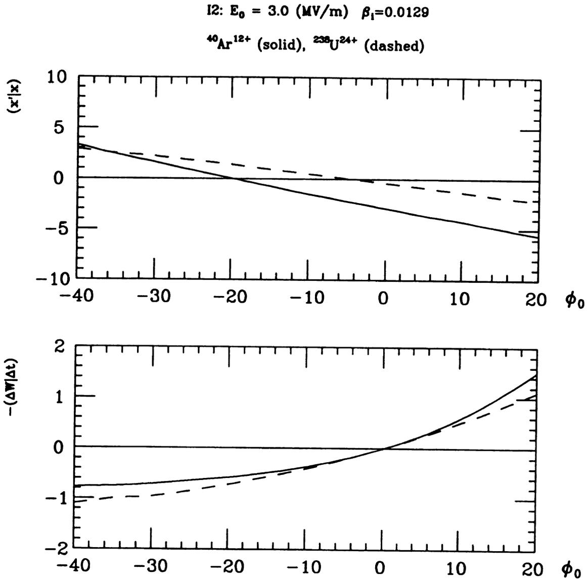
Figure 4.10: The plots of  $(x'|x)$  and  $-(\Delta w/\Delta t)$  vs. rf phase offset  $\phi_0$  for an I2 type resonator. The solid line is for  $^{40}\text{Ar}^{12+}$  with  $\beta_i = 0.0164$  and the dashed line is for  $^{238}\text{U}^{24+}$  with  $\beta_i = 0.0164$ .
