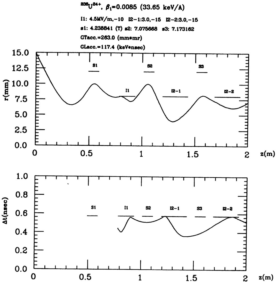
Figure 5.8: The beam envelopes of beam radius (upper) and deviation of time of flight (lower) starting with a maximum emittance in the system using solenoids for the transverse focusing. The incident velocity of the  $^{238}\text{U}^{24+}$  beam was 0.0085c.
