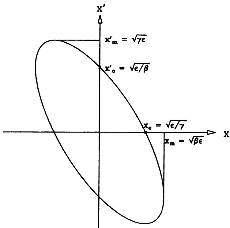
Figure 2.1: A two dimensional beam phase space ellipse. The equation of the ellipse is given by  $\gamma x^2 + 2\alpha x x' + \beta x'^2 = \epsilon$ . The area of the phase space ellipse is  $\pi\epsilon$ . The  $\epsilon$  is called beam emittance.
