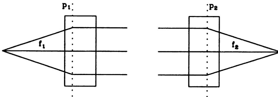
Figure 4.1: The point-to-parallel system(left) and the parallel-to-point system(right).  $P_1$  and  $P_2$  are two different principal planes.
