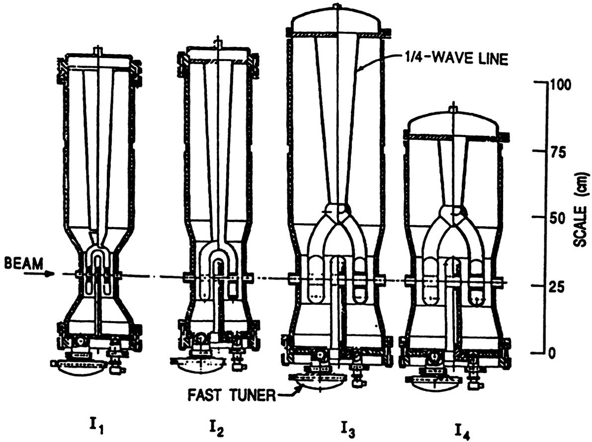
Figure 1.3: The resonators of the PII linac.
