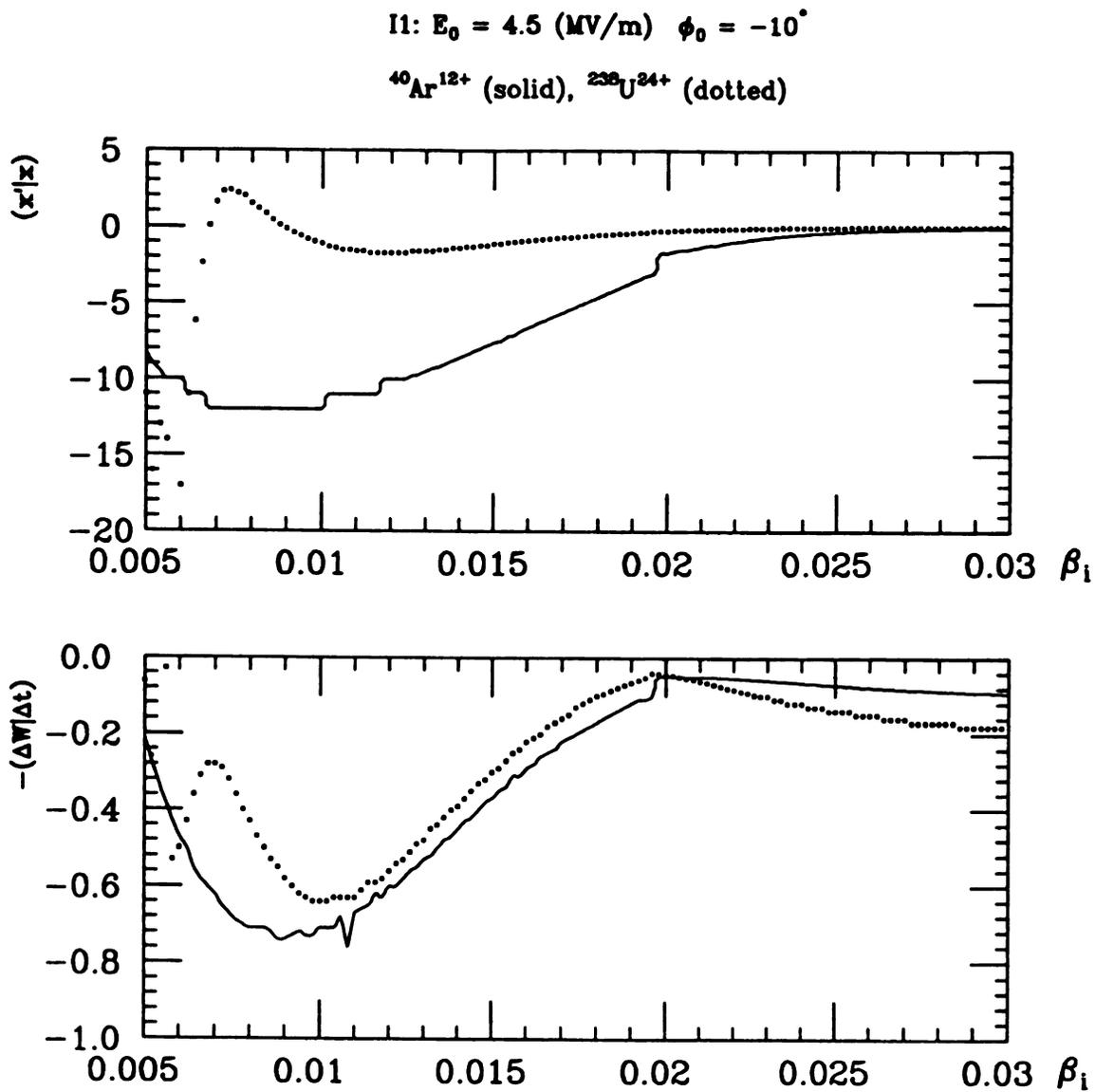
Figure 4.7: The plots of  $(x'|x)$  and  $-(\Delta w|\Delta t)$  vs. initial beta  $\beta_i$  for an I1 type resonator. The solid line is for  $^{40}\text{Ar}^{12+}$  and the dotted line is for  $^{238}\text{U}^{24+}$ .
