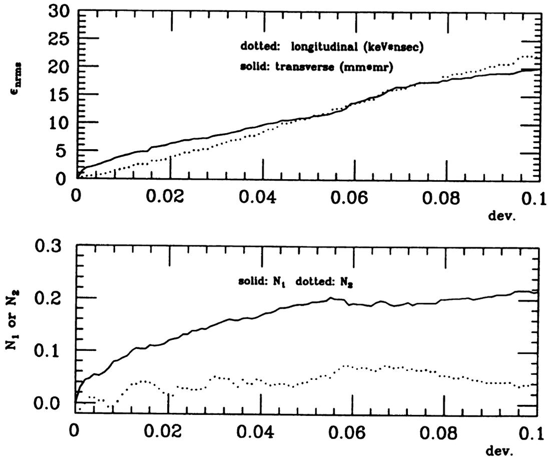
Figure 5.6: The relationship between scalings of nonlinearity by linear transformation and by rms emittance for a  $^{238}\text{U}^{24+}$  beam with an incident velocity  $0.007c$ . The initial geometrical transverse acceptance was  $140.49 \text{ mm} \cdot \text{mr}$  without longitudinal phase space.
