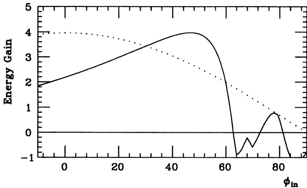
Figure 1.4: The curve of energy gain versus incident rf phase angle of type II resonator. The dotted line is the typical energy gain curve of a high beta resonator (not scaled).
