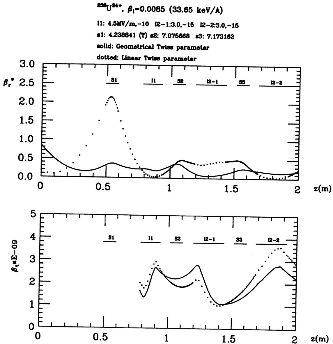
Figure 5.13: The effective beta-functions of the transverse (upper) and the longitudinal (lower) phase spaces for  $^{238}\text{U}^{24+}$  beam with an incident velocity  $0.0085c$  in the system using solenoids for the transverse focusing. The dotted lines are for Twiss parameters from the geometrical acceptances and the solid line is for Twiss parameters from the linear acceptances.
