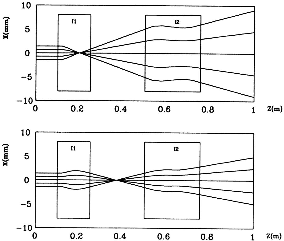
Figure 4.13: The transverse raytracing plots for  $^{40}\text{Ar}^{12+}$  (up) and  $^{238}\text{U}^{24+}$  (down) beams with parallel rays at the beginning.
