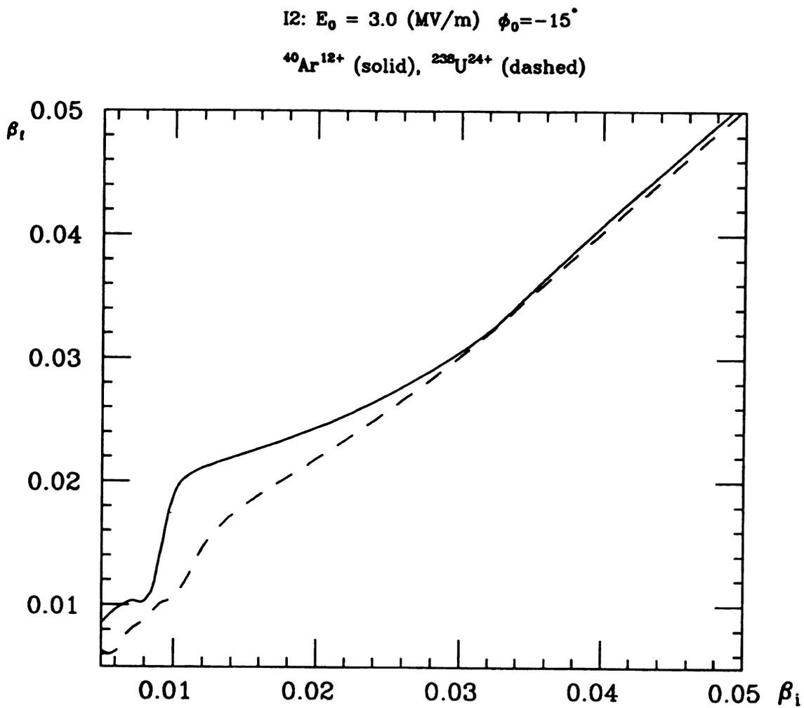
Figure 4.12: The plot for initial beta  $\beta_i$  vs. final beta  $\beta_f$  of I2 type resonator. The solid line is for  $^{40}\text{Ar}^{12+}$  and dashed line for  $^{238}\text{U}^{24+}$  beam.
