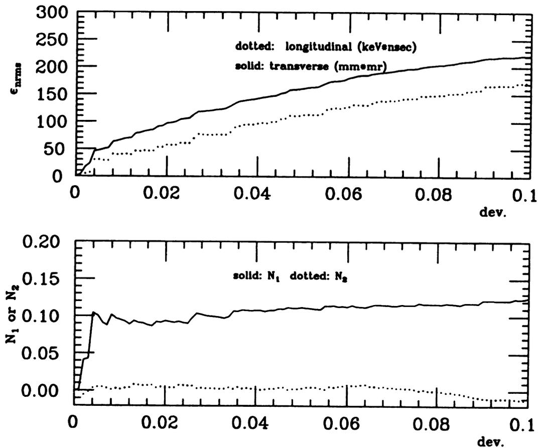
Figure 5.11: the relationship between scalings of nonlinearity by linear transformation and by rms emittance for a  $^{238}\text{U}^{24+}$  beam with an incident velocity 0.0085c in the system using solenoids for transverse focusing. The initial geometrical transverse acceptance was 263 mm·mr without longitudinal phase space.
