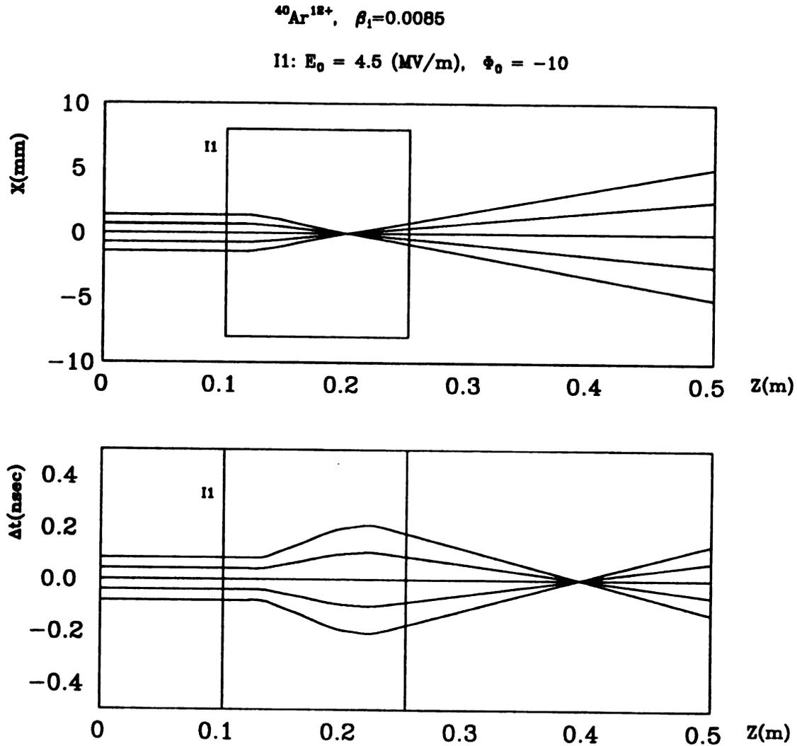
Figure 1.11: The transverse (upper) and longitudinal (lower) focusing properties of type II resonator for  $^{40}\text{Ar}^{12+}$  beam with incident velocity  $0.0085c$ . The amplitude of electric field gradient and initial rf phase angle were  $4.5$  MV/m and  $-10$  degrees respectively.
