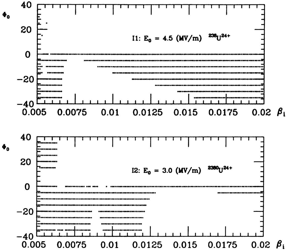
Figure 4.6: The stability region of the rf phase offset of I1 (up) and I2 type (down) resonators as a function of initial  $\beta$  for  $^{238}\text{U}^{24+}$  beam.
