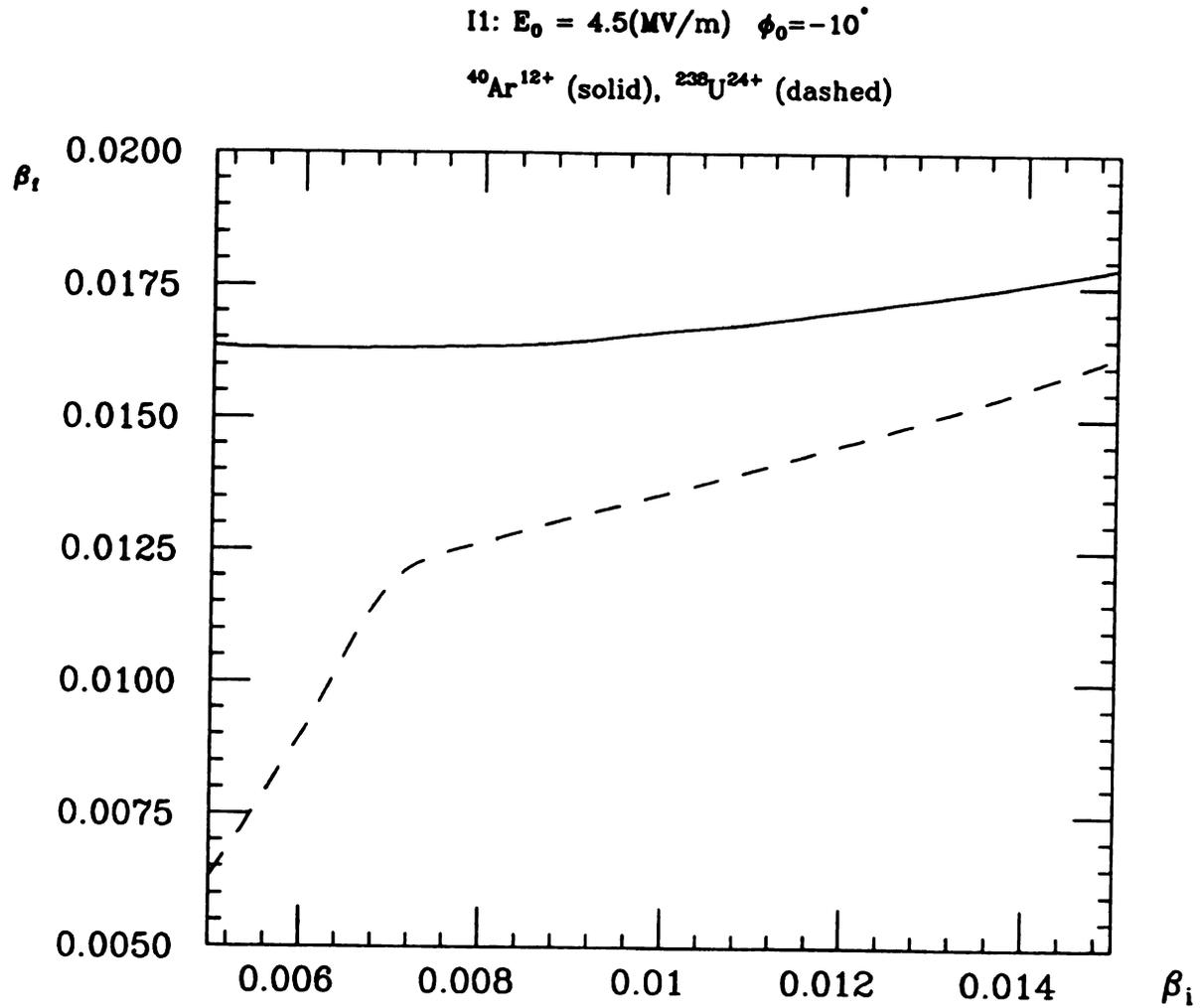
Figure 4.11: The plot for initial beta  $\beta_i$  vs. final beta  $\beta_f$  of an I1 type resonator. The solid line is for  $^{40}\text{Ar}^{12+}$  and the dashed line for  $^{238}\text{U}^{24+}$  beam.
