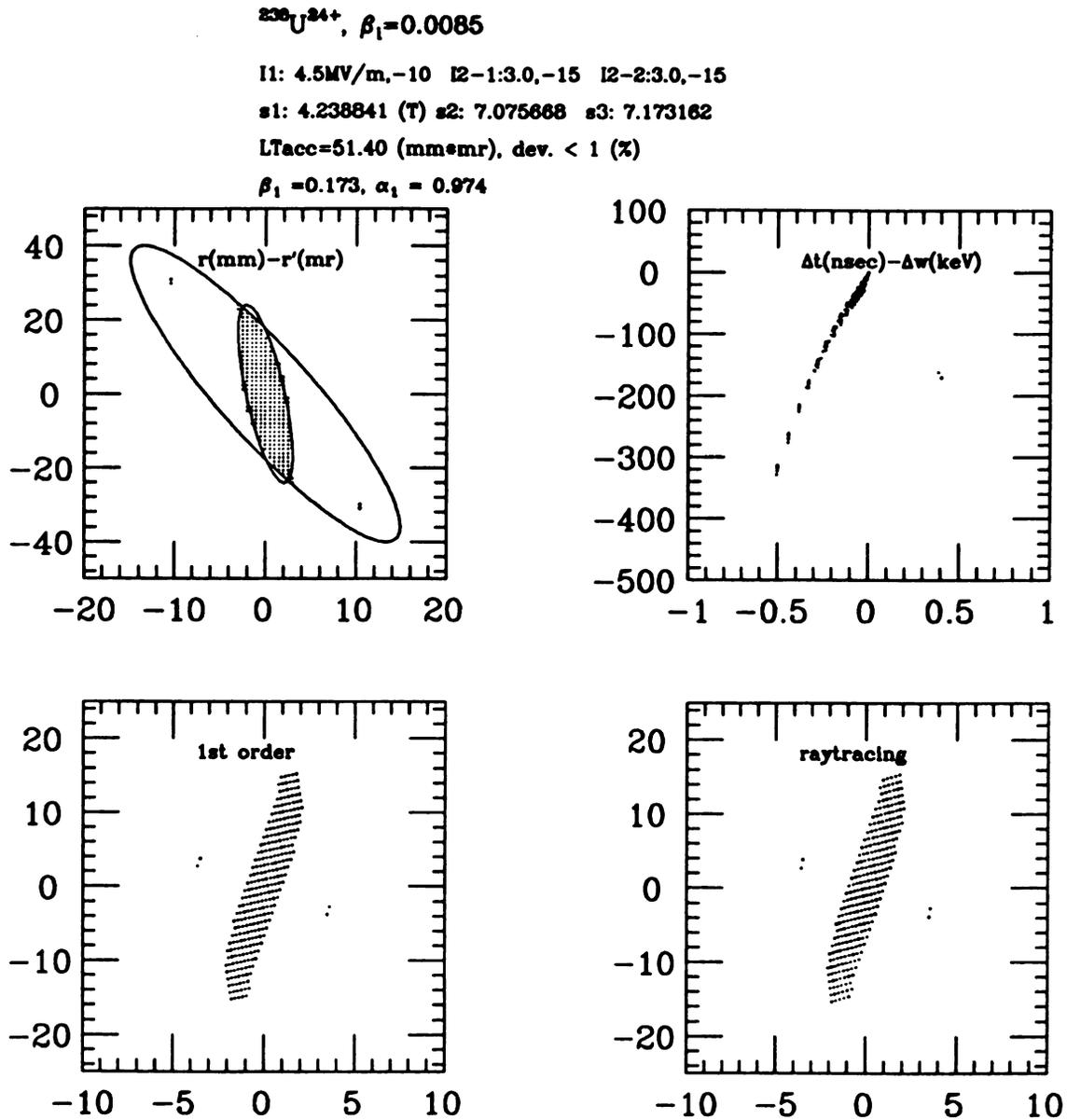
Figure 5.9: The phase space transformations of the transverse linear acceptance in the system using solenoids for the transverse focusing. The incident velocity of the  $^{238}\text{U}^{24+}$  beam was  $0.0085c$ .
