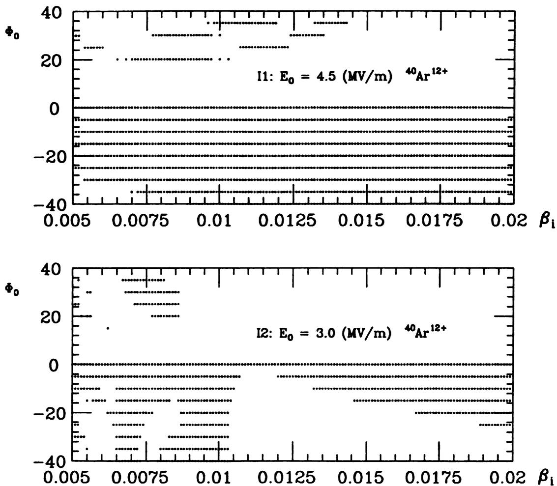
Figure 4.5: The stability region of the rf phase offset of I1 (up) and I2 type (down) resonators as a function of initial  $\beta$  for  $^{40}\text{Ar}^{12+}$  beam.
