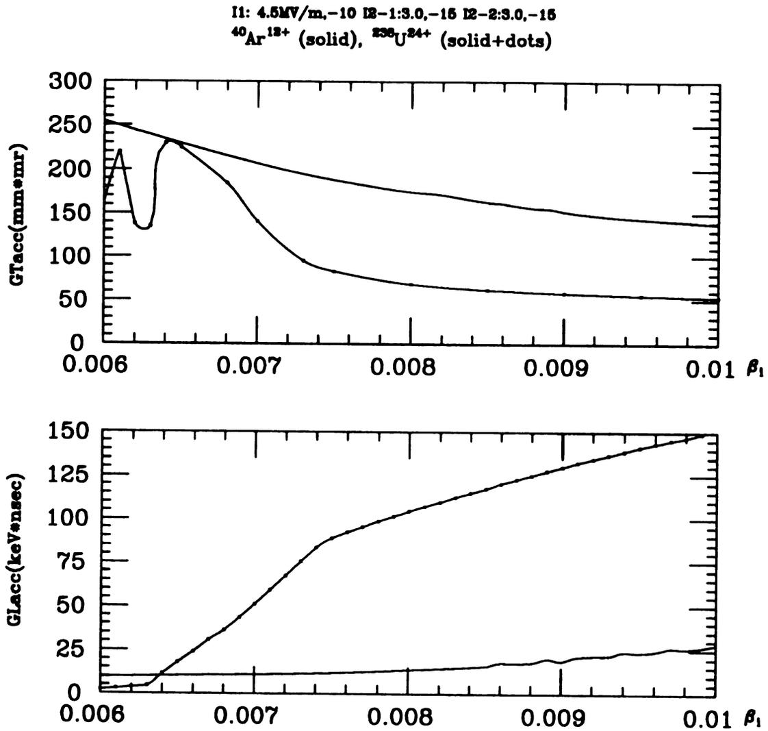
Figure 5.1: The geometrical transverse (upper) and longitudinal (lower) acceptances as a functions of incident velocities.
