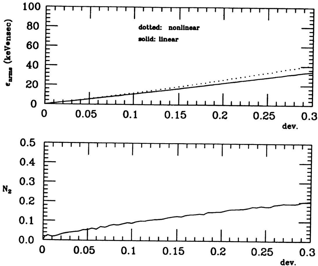
Figure 5.7: The relationship between scalings of nonlinearity by linear transformation and by rms emittance for a  $^{238}\text{U}^{24+}$  beam with an incident velocity  $0.007c$ . The initial geometrical longitudinal acceptance was  $51.07 \text{ keV} \cdot \text{nsec}$  without transverse phase space.
