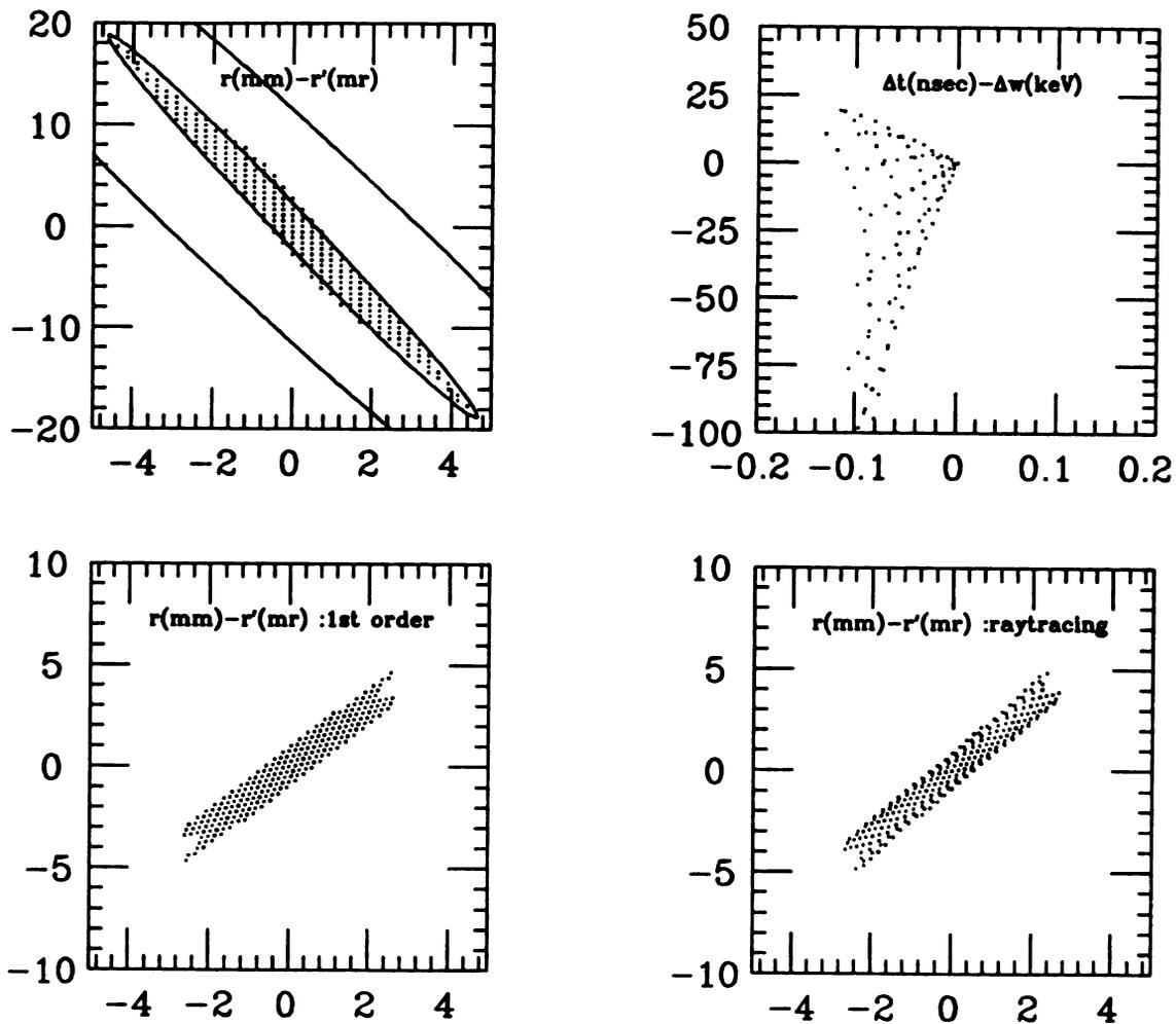
Figure 5.4: The phase space transformations of the transverse linear acceptance for a  $^{238}\text{U}^{24+}$  beam with an incident velocity  $0.007c$  with a deviation of 5%.
