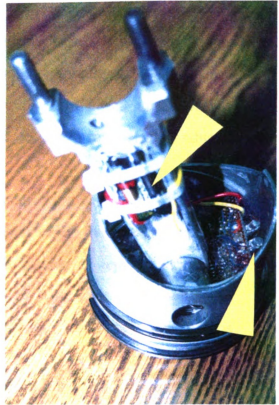
Figure 2 : Piston with Rod: Telemetry Board with IR-Diodes within the Piston and Batteries on the ConnectingRod (see arrows)
