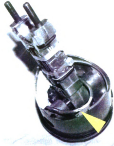
Figure 17: Teflon- and Silver shielded Power Supply Cable with Wear after Main Test Run
