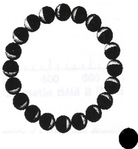
Figure 5.7: Rings of 20 magnetic dipoles in an external field which is (a) parallel (300 G) and (b) perpendicular (500 G) to the ring plane. The external field is represented by the arrows, and has the same coloring convention as the magnetic dipoles, used in Fig. 5.4.
