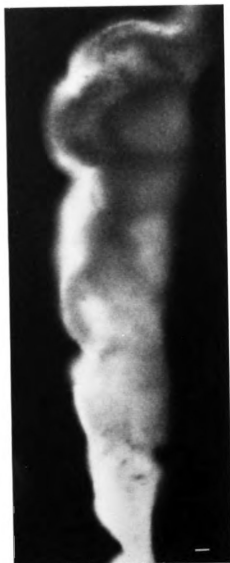
Figure 10. Laser scanning dark field photomicrograph of a 77-day-old bacterial GAC coated particle showing variation of the biofilm thickness within the same colonized surface. Bar, 30 \mu\text{m} .
