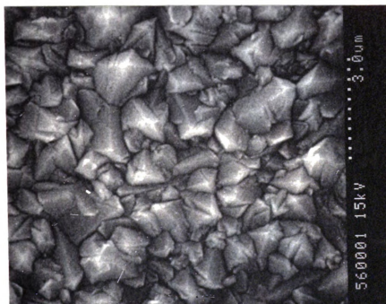
Figure A7. The deposition surface of DF-N5-6. The surface is dominated by (111) facets. A grain size of 0.64 micron was determined from this micrograph. A 3.0 micron dot-bar is indicated.
