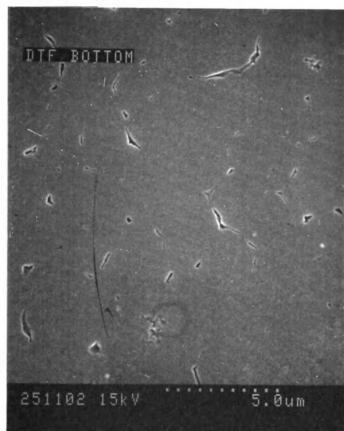
Figure 22 (a). Micrograph of the interfacial surface of the DTF specimen WF#25-11 showing distinct grain boundaries defined by the dark lines. A grain size of 0.71 micron was determined from this micrograph. The dotted bar represents 5 microns.
