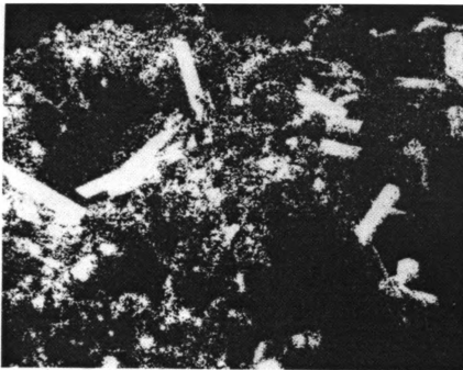
Figure 2.10 - Energy dispersive x-ray spectroscopy fractograph showing the distribution of sulfur in asphalt at 118X [45].
