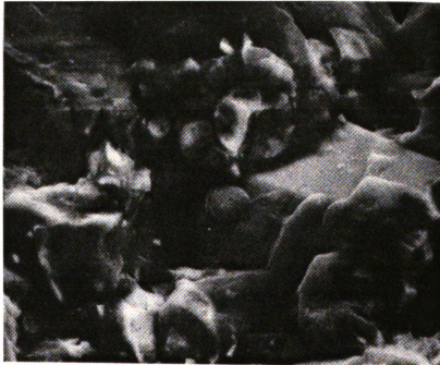
Figure 2.13 - Backscattered electron fractograph of sulfur modified asphalt showing the morphology of the crystalline sulfur at 1176X [45].
