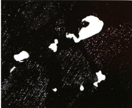
Figure 5.5 - Micrograph using reflected light through an optical microscope showing voids in a good sample at 41X.
