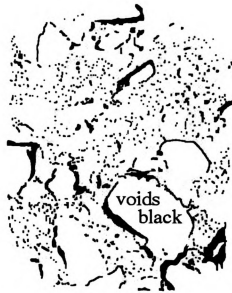
Figure 5.20 - Illustration of Bad150 showing the voids at 1.2X.
