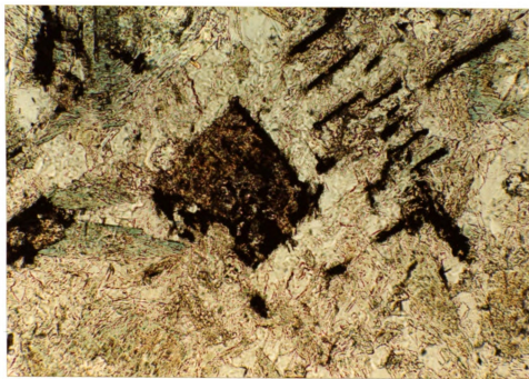
Figure 13.--Photomicrograph of altered pyroxene, with significant alteration to opaque minerals. Surrounding grains display remnant igneous textures.
