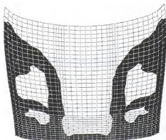
Figure 5.38. Example 4: Interpretation of the optimum shape of the car hood.
