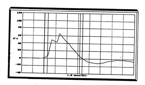
Figure 5: Shock Pulses for Double Impacts
