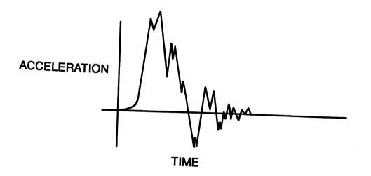
Figure 2: Acceleration Time History of a Mechanical Shock
