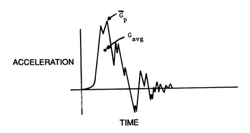
Figure 8: Acceleration Time Plot Representing Pallet Marshalling Impacts
