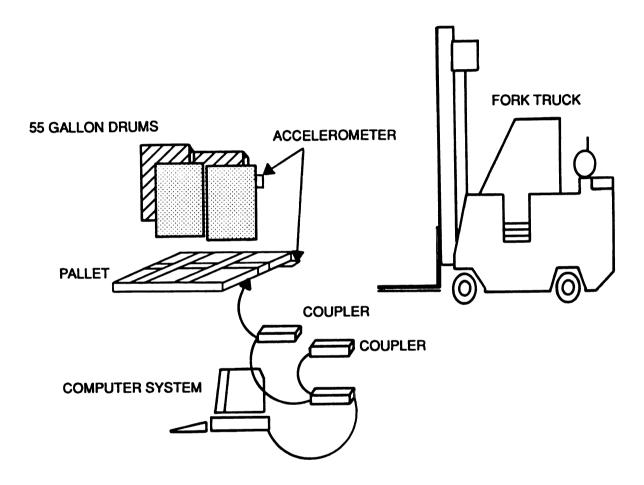
Figure 3: Test Setup to Measure Pallet Impacts
