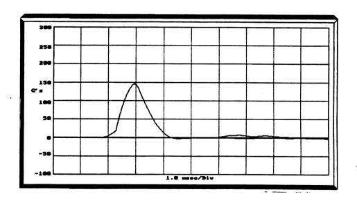
Figure 6: Shock Pulses for Good Impacts
