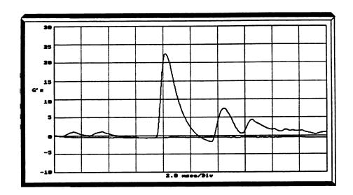
Figure 4: Shock Pulses for Multiple Impacts
