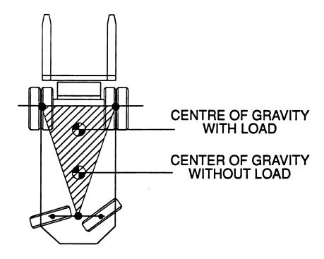
Figure 1: Stability Polygon of a 4 Wheel Truck
