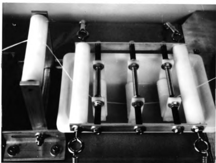
Figure 36. Cradle-roller guide and suspension bath assembly.
