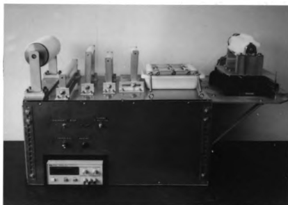
Figure 34. 35mm photograph showing the various components of the laboratory-scale FED filament winding system.
