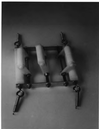
Figure 37. Rotational motion of cradle-roller assembly.
