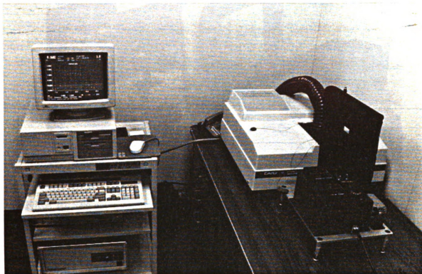
FIGURE 9: Setup for determining vapor concentration.
