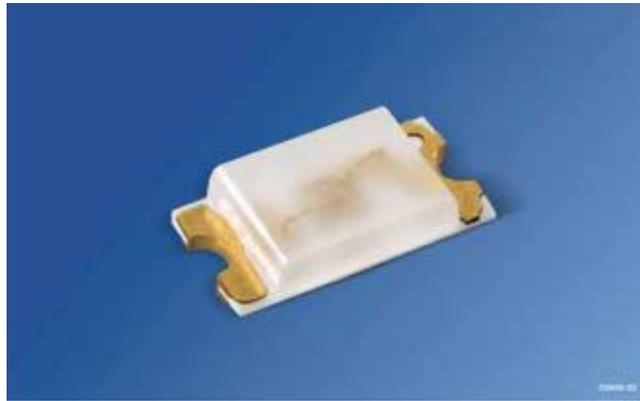
*Figure 5* The LED used in the experiment. It is packaged with a colorless diffused resin.
