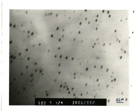
Figure 5-3 Morphology of blend after annealing 5 minutes at 180°C as viewed in plane of extrudate strand axis
