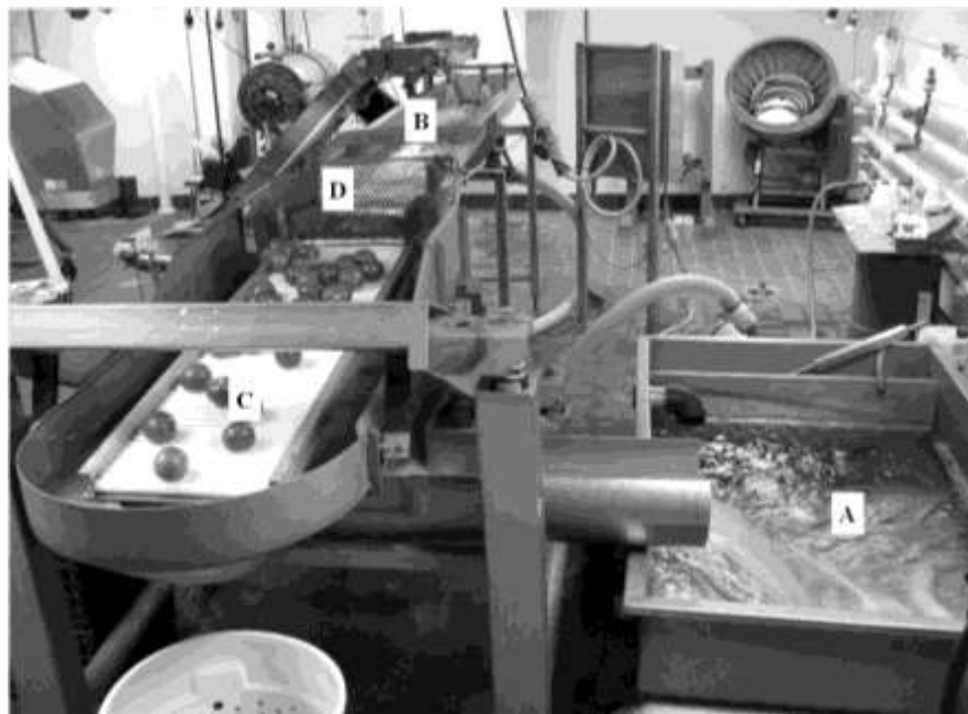
Figure 3.2: Pilot-scale tomato processing line: (A) water tank, (B) dump tank, (C) roller conveyor, and (D) stainless steel retention screen.
