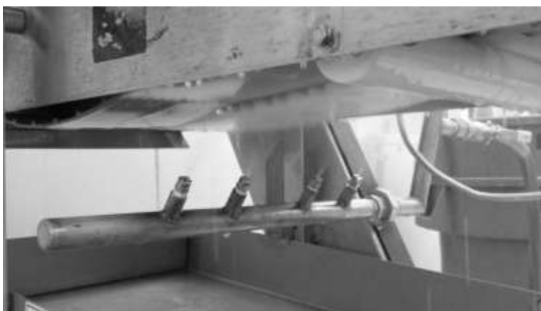
Figure 6.3: Dual belt conveyor system: (A) smooth (left) and interlocking (right) belt, (B) inoculation tray, (C) spray bar.
