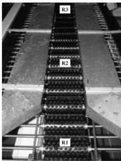
Figure 4.2: Three types of roller conveyor: (A) plastic, (B) foam, and (C) brush roller conveyor.
